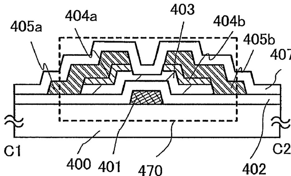
semiconductor layer including a channel formation region using an oxide semiconductor layer, a source region, and a drain region are formed using an oxide semiconductor layer, heat treatment for reducing impurities such as moisture (heat treatment for dehydration or dehydrogenation) is performed so as to improve the purity of the oxide semiconductor layer.
