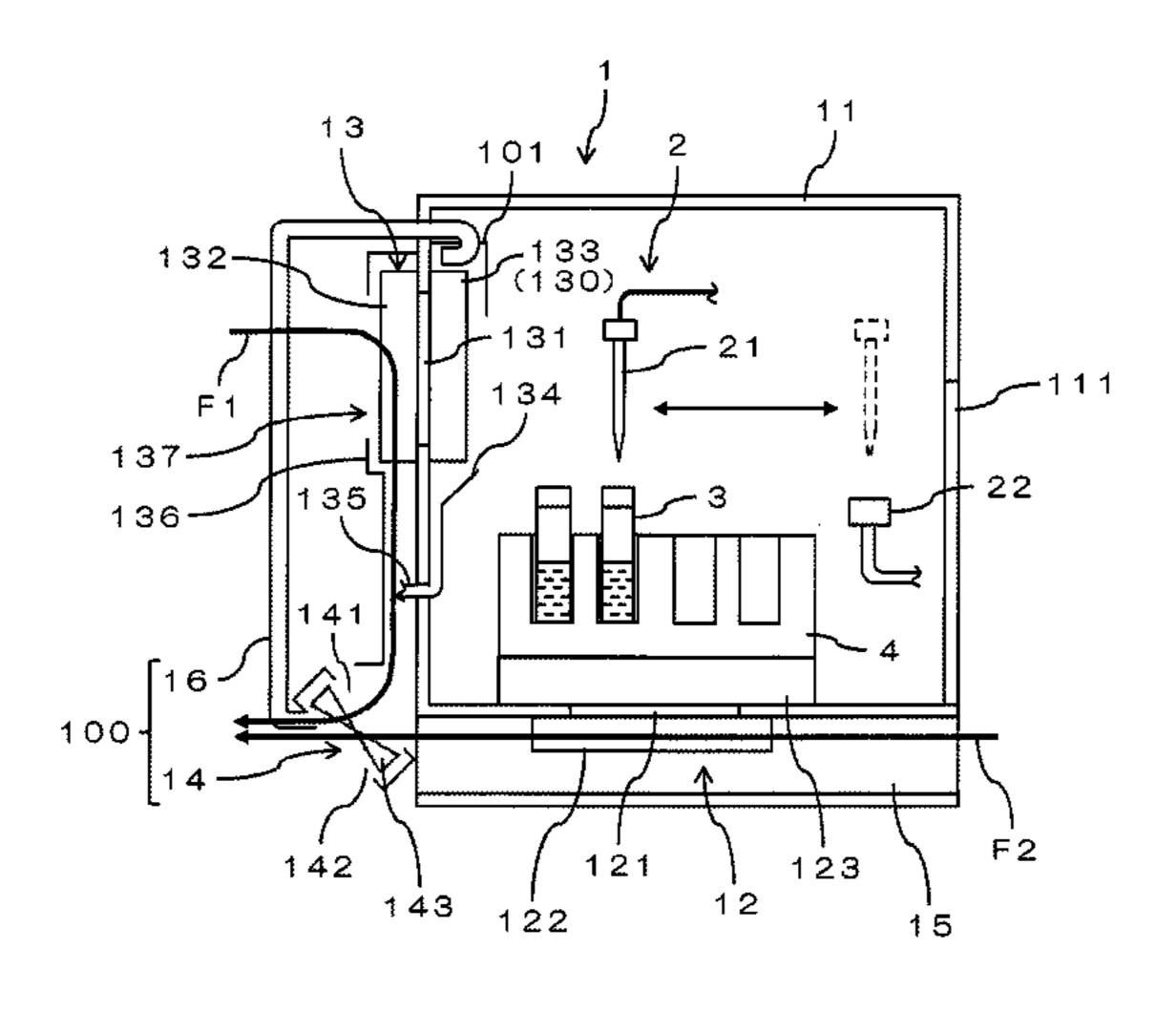
fier section 13, the humidity inside the accommodating chamber 11 may be prevented from rising due to the air that is sent from the blower section 100.
