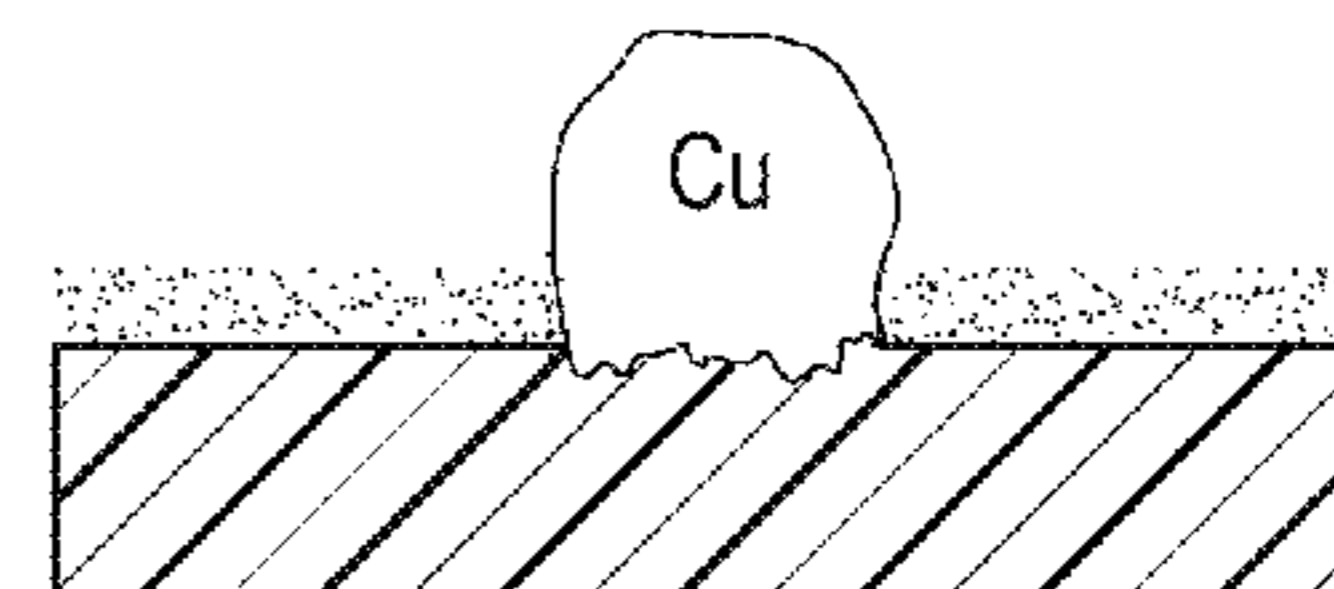
5. Metallization by electroless copper • Electroless copper reaction is initiated at the LDS area which covered by active catalyst
