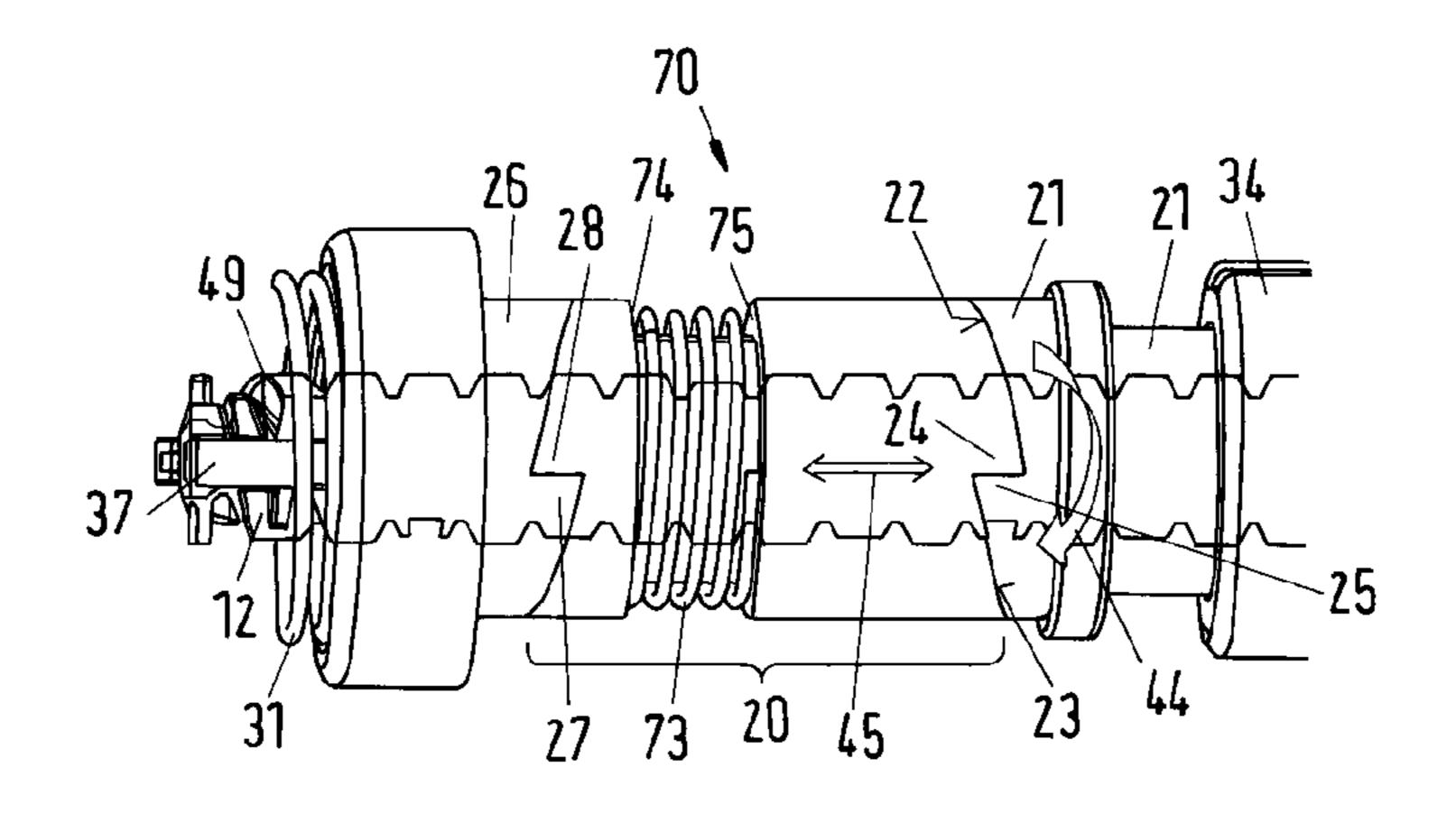
relative rotational movement of the first and second drive parts is prevented and relative axial movement is permitted.
