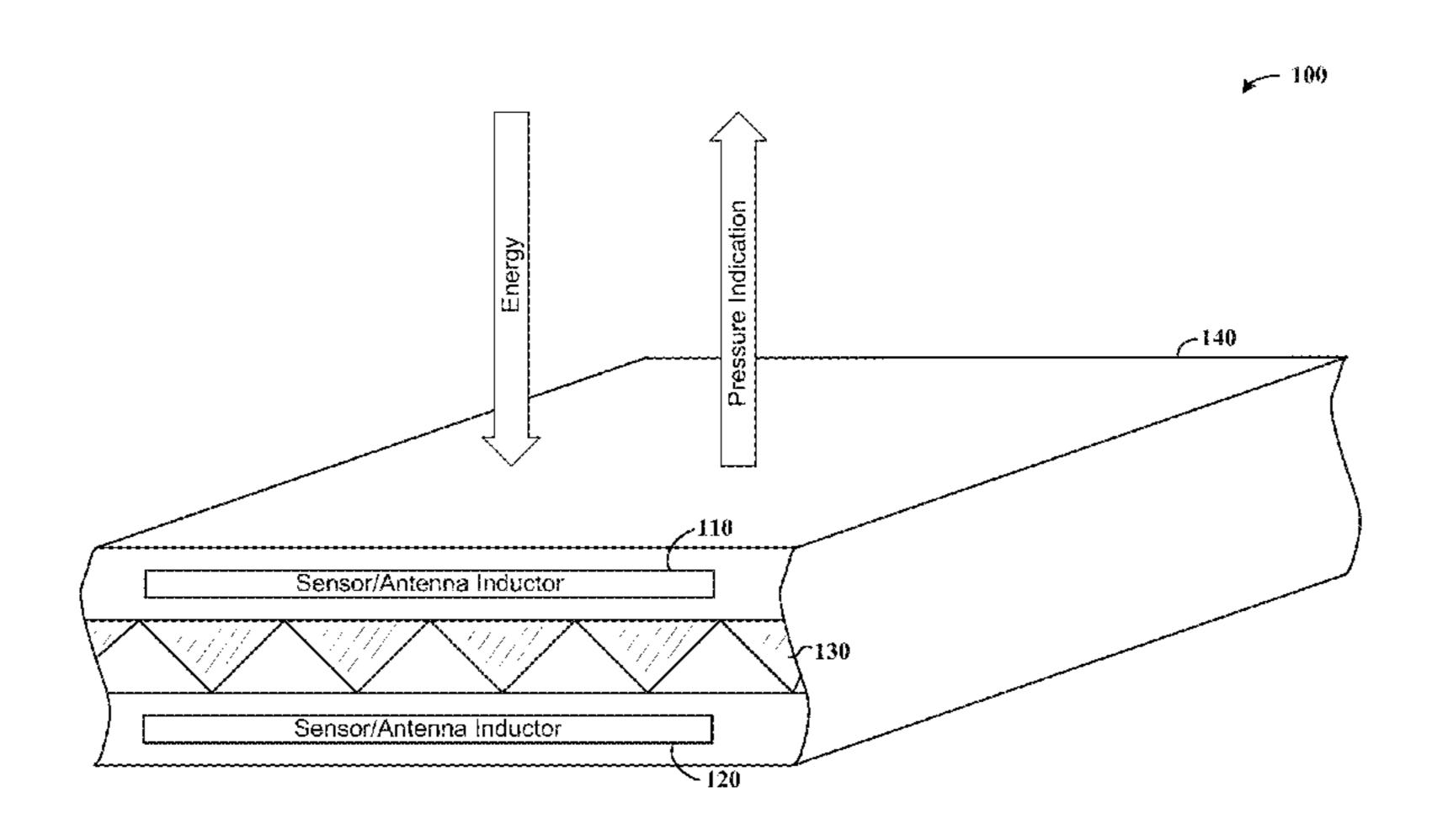
These resonant frequencies, or a change in the resonant frequencies, can be used as an indication of the pressure.
