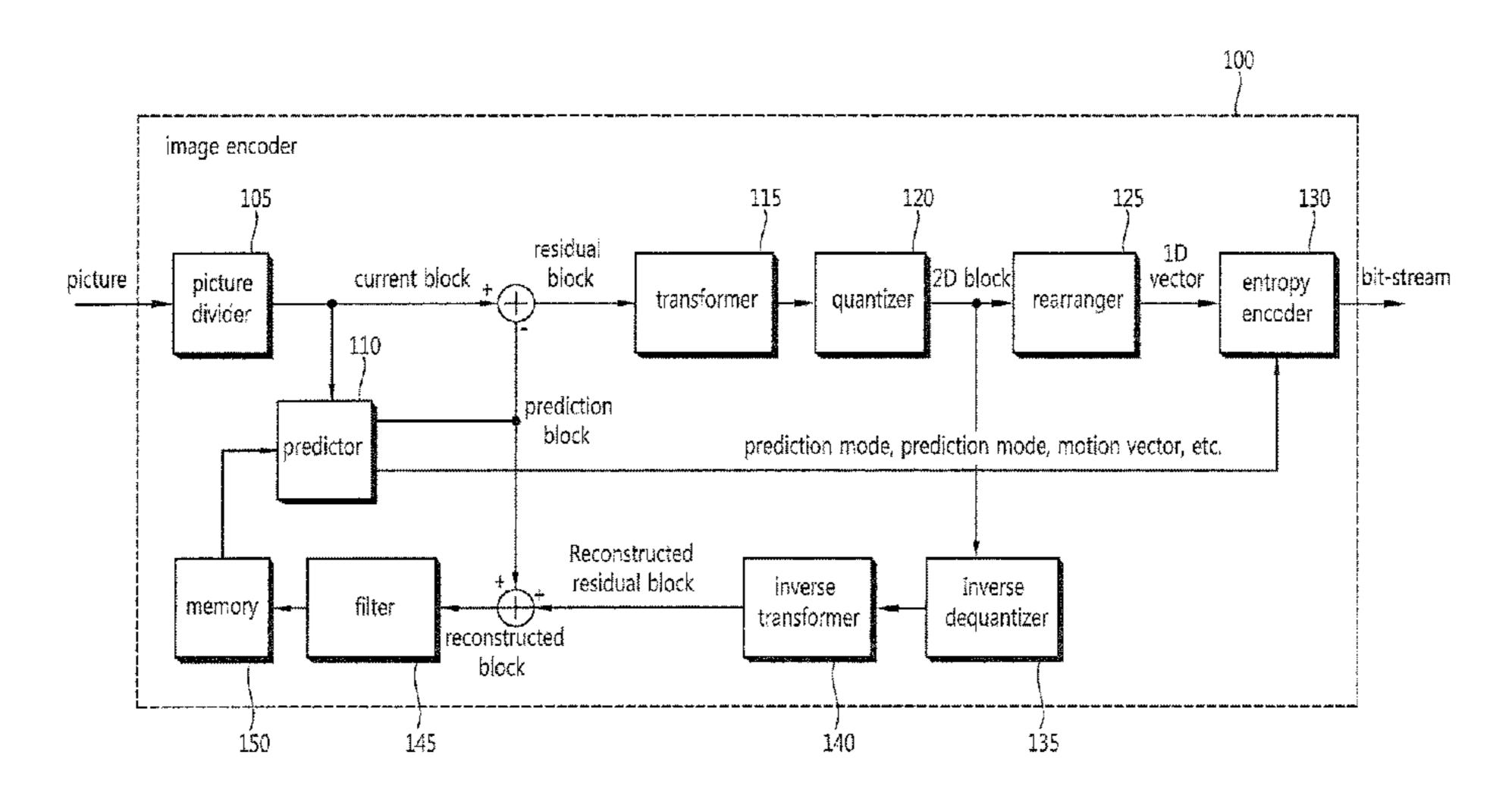
prediction mode to generate a prediction block corresponding to the current block.
