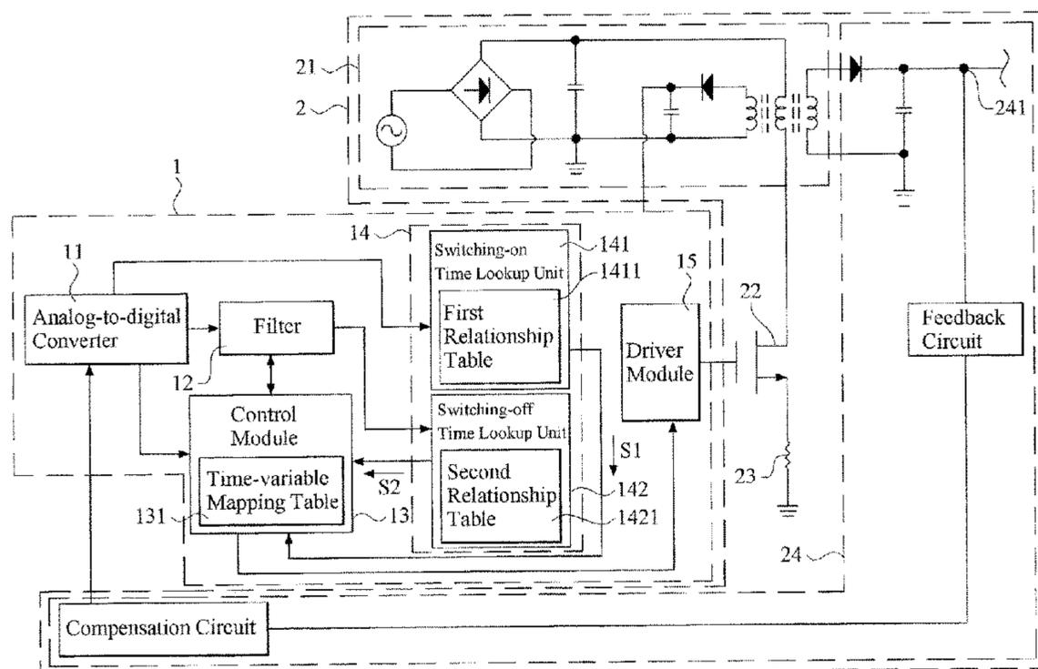
switch. While the control module detects that the load status switches to a heavy-load status and the voltage difference reaches the threshold voltage, the control duty cycle is increased. While the control module detects that the load status switches to the light-load status and the voltage difference reaches the threshold voltage, the control duty cycle is decreased.
