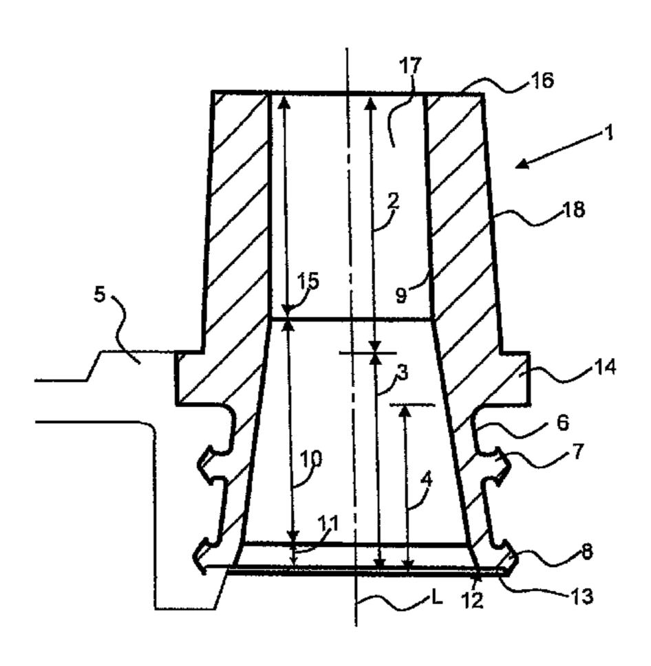
ferential projection (7, 8). Also disclosed is a rechargeable battery housing or a part of said rechargeable battery housing having at least one connecting pole.
