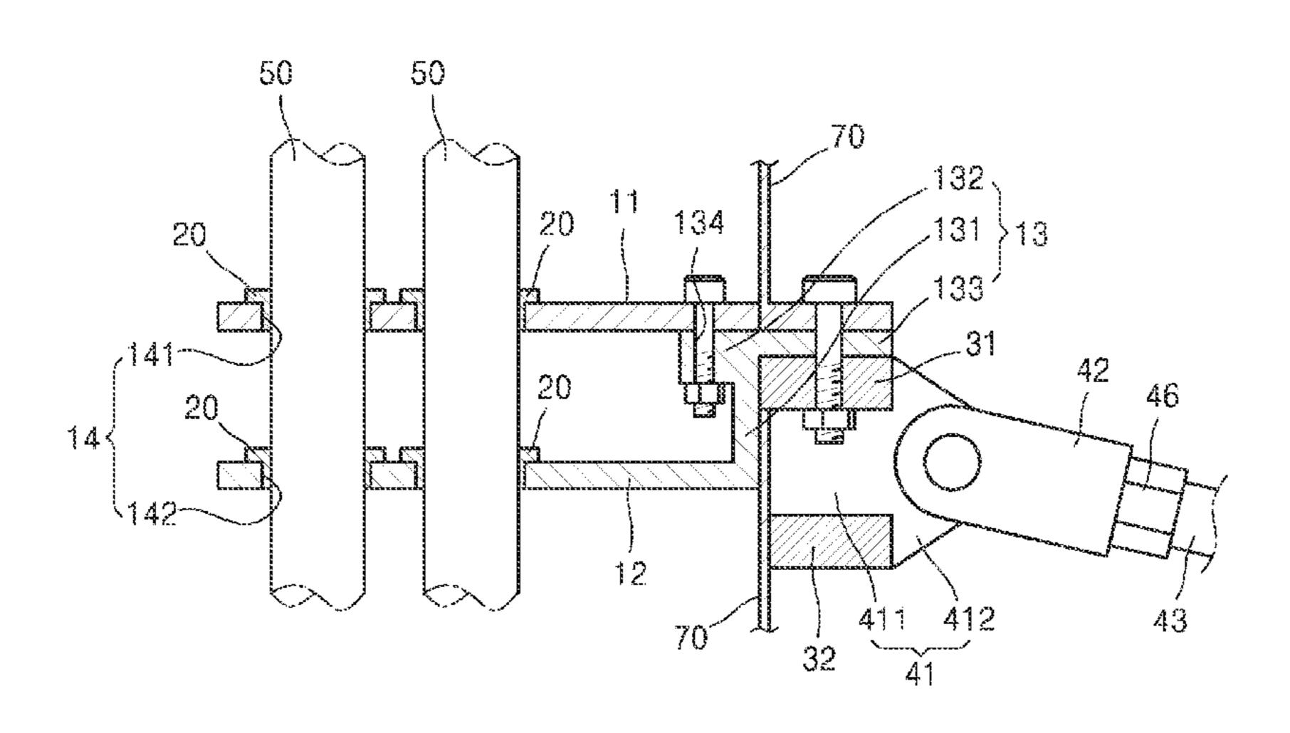
and a connection part connecting the upper support plate and the lower support plate. The connection part includes a support beam vertically extending from an end portion of the lower support plate, an inner flange extending inward from an upper end portion of the support beam, and an outer flange extending outward from the upper end portion of the support beam.
