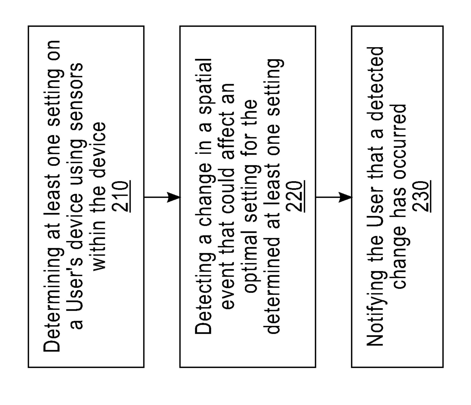
Determining at least one setting on a User's device using sensors within the device
