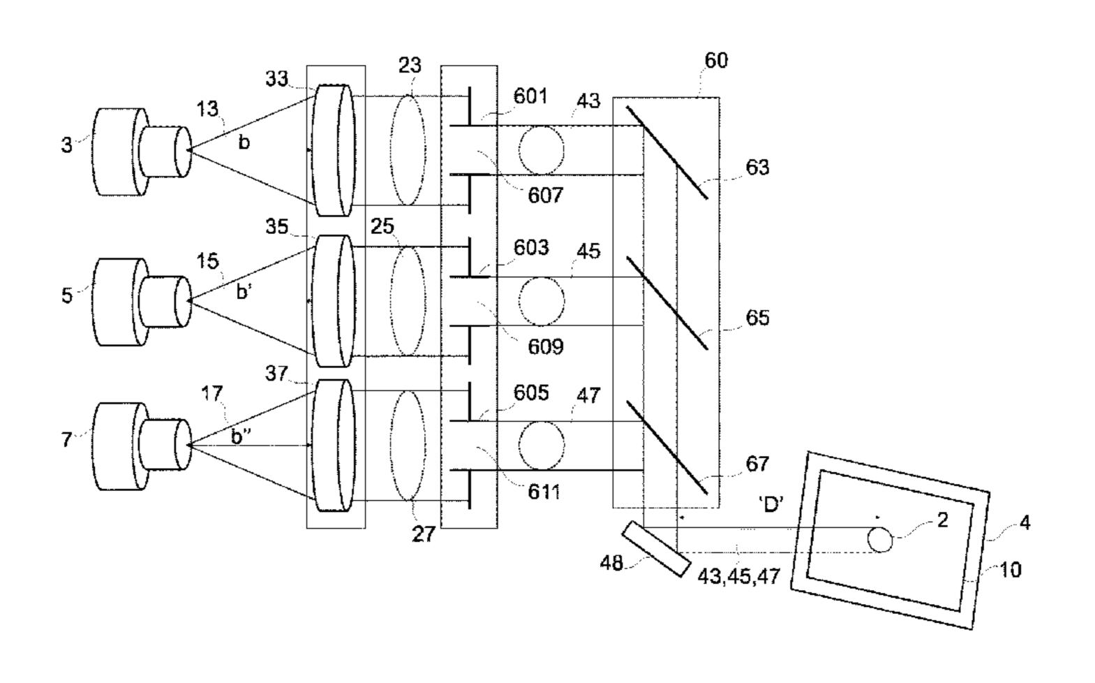
ured such that it can oscillate about at least one oscillation axis to scan the red, green and blue projection beams across a projection screen which is positioned at the predetermined distance from the projection device.
