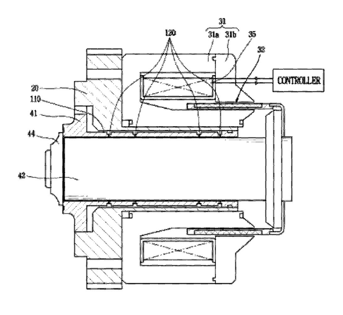
noise generated when a refrigerant is discharged in the compression space. Furthermore, the number of vibrations of a mover is increased and a driving operation for removing foreign substances is carried out to increase the number of vibrations of a cylinder such that any foreign substance stuck in a gas hole can be cleaned, thereby increasing performance and reliability of the compressor.
