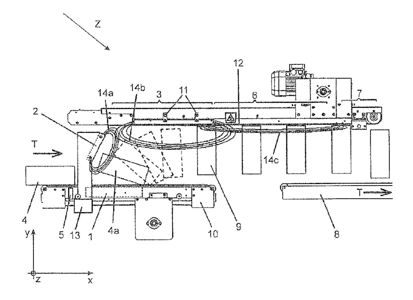
position hanging magnetically at the transport device (12). The control device (13) is adapted to activate the first magnet arrangement (1) when a front edge of a body (4) lying on the input transport device (10) has passed the second magnet arrangement (2) and to deactivate the first magnet arrangement (1) when a trailing edge of this body (4) comes to lie below the second magnet arrangement (2).
