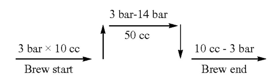
and the third dispensing step achieves a post-infusion in which said hydraulic pump is deactivated for a time needed to reach by weight the programmed dose of product dispensed.
