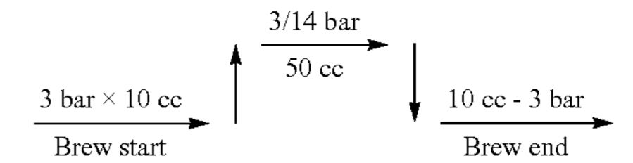
The method allows, by controlling the quantity by volume of water calculated to achieve a desired brew ratio, to enhance the extraction of the aromas and all the organoleptic qualities during the dispensing of the espresso coffee, once the weight of the coffee in the cup 15 has been measured with respect to the weight of the coffee powder contained in the filter basket holder 5.
