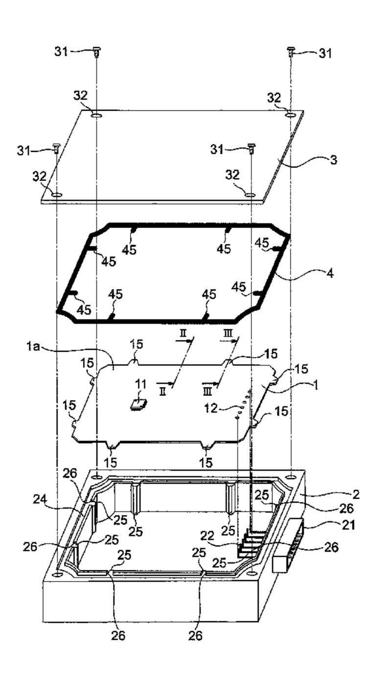
screws (31) so that a packing main body (4a) hermetically seals an inside of the housing. Packing projecting portions (45) of the rubber packing (4) press circuit-board protruding portions (15), to thereby hold the printed circuit board (1) inside the housing.
