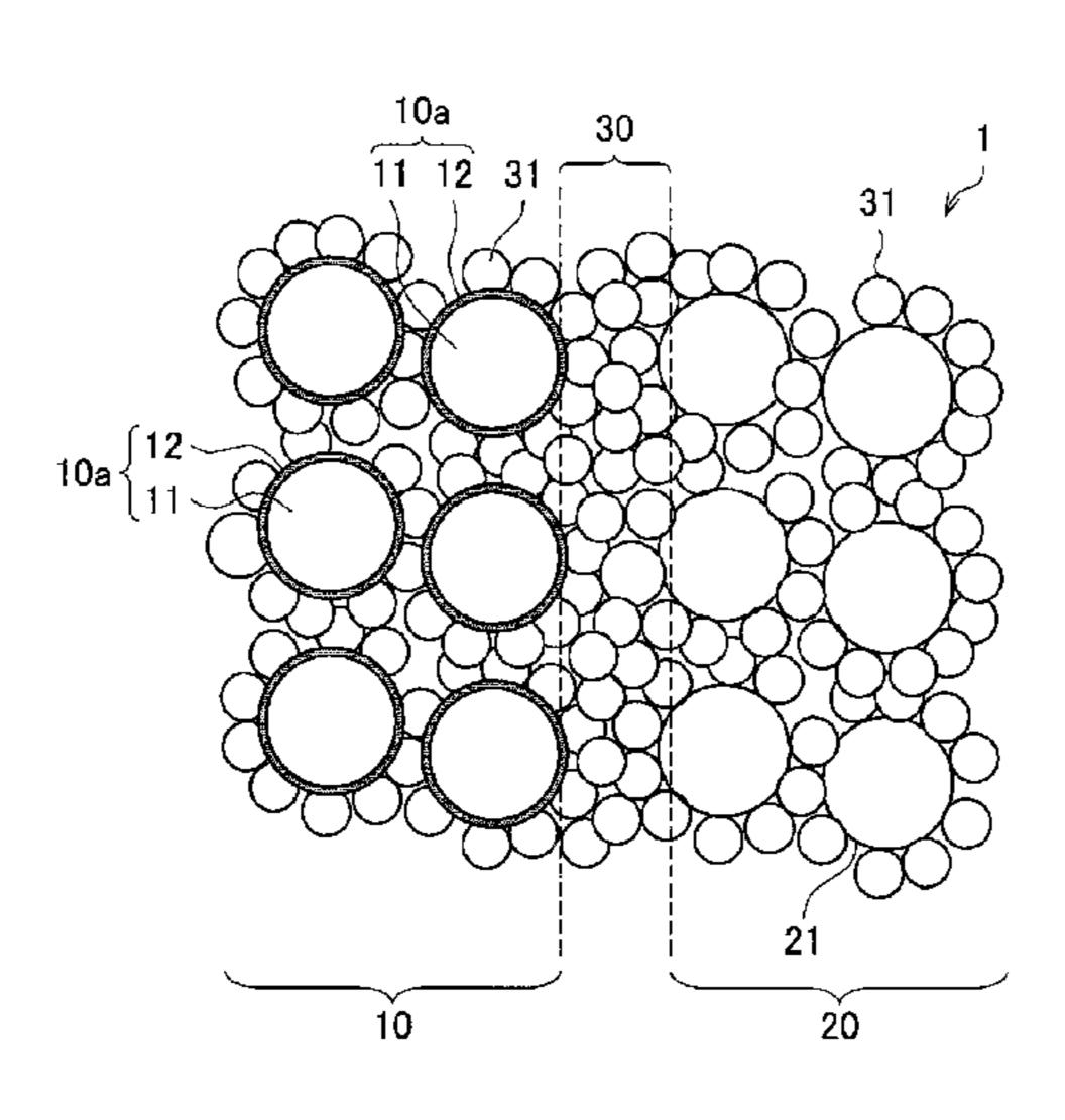
a ratio of a thickness of the reactive layer to a particle diameter of the positive active material particle is in a range of about 0.0010 to about 0.25.
