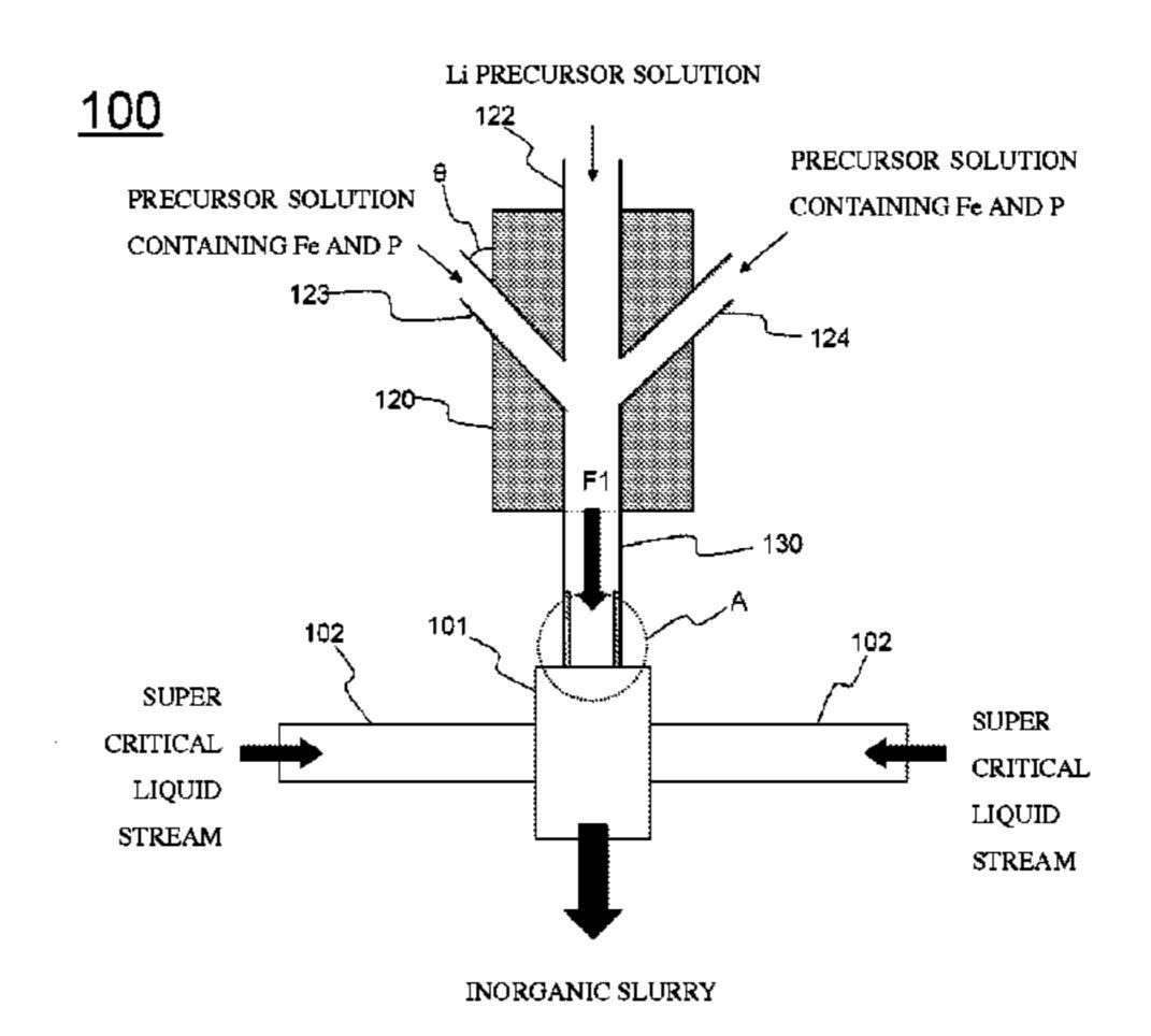
to the connection tube into which the intermediate slurry prepared from the mixer is introduced and to at least one injection tube into which the heated liquid stream is injected.
