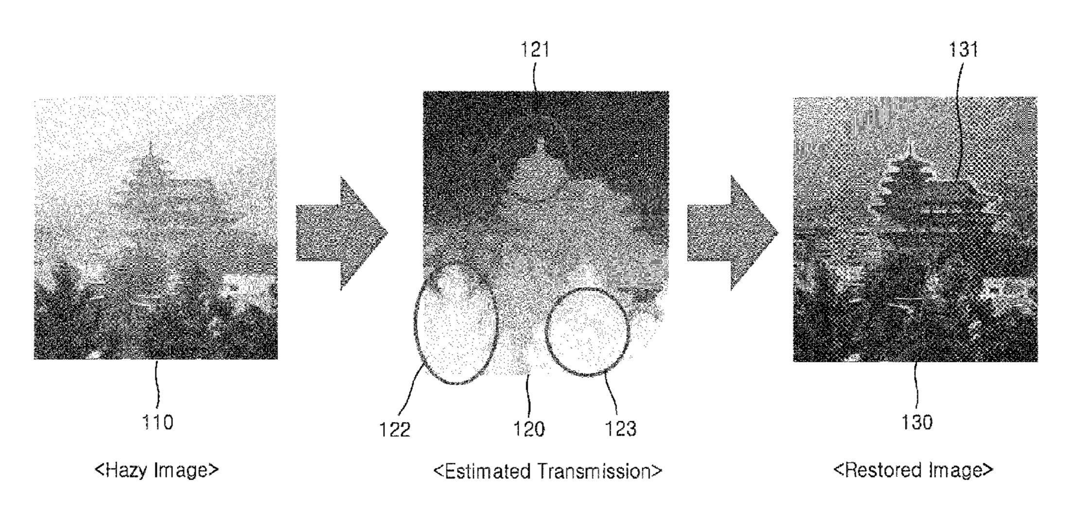
restored based on the refined transmission value, and then multi-scale tone manipulation image processing is performed.
