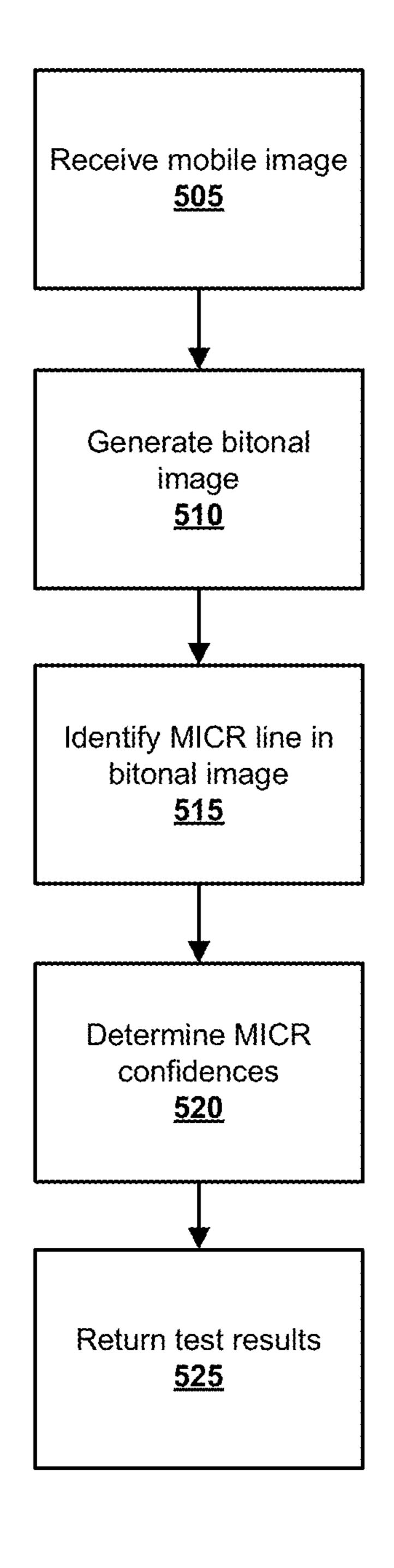
FIG. 5 MICR-line Test
