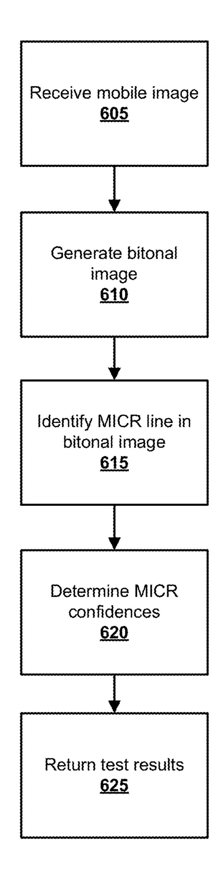
FIG. 6 Front-as-Rear Test
