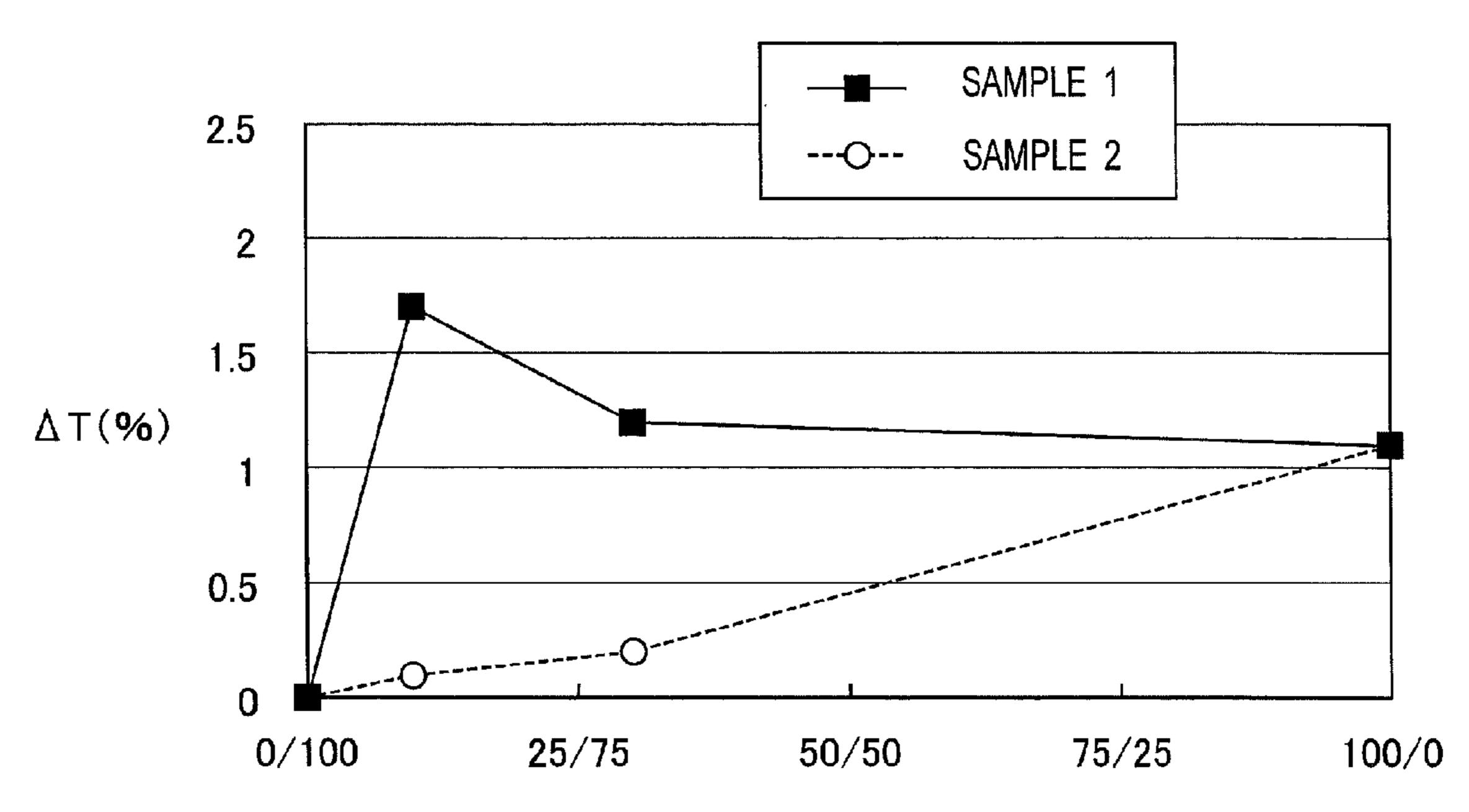
MASS RATIO OF FLUORORESIN TO HYDROXYL GROUP-CONTAINING ACRYLIC RESIN (FLUORORESIN / HYDROXYL GROUP-CONTAINING ACRYLIC RESIN)
