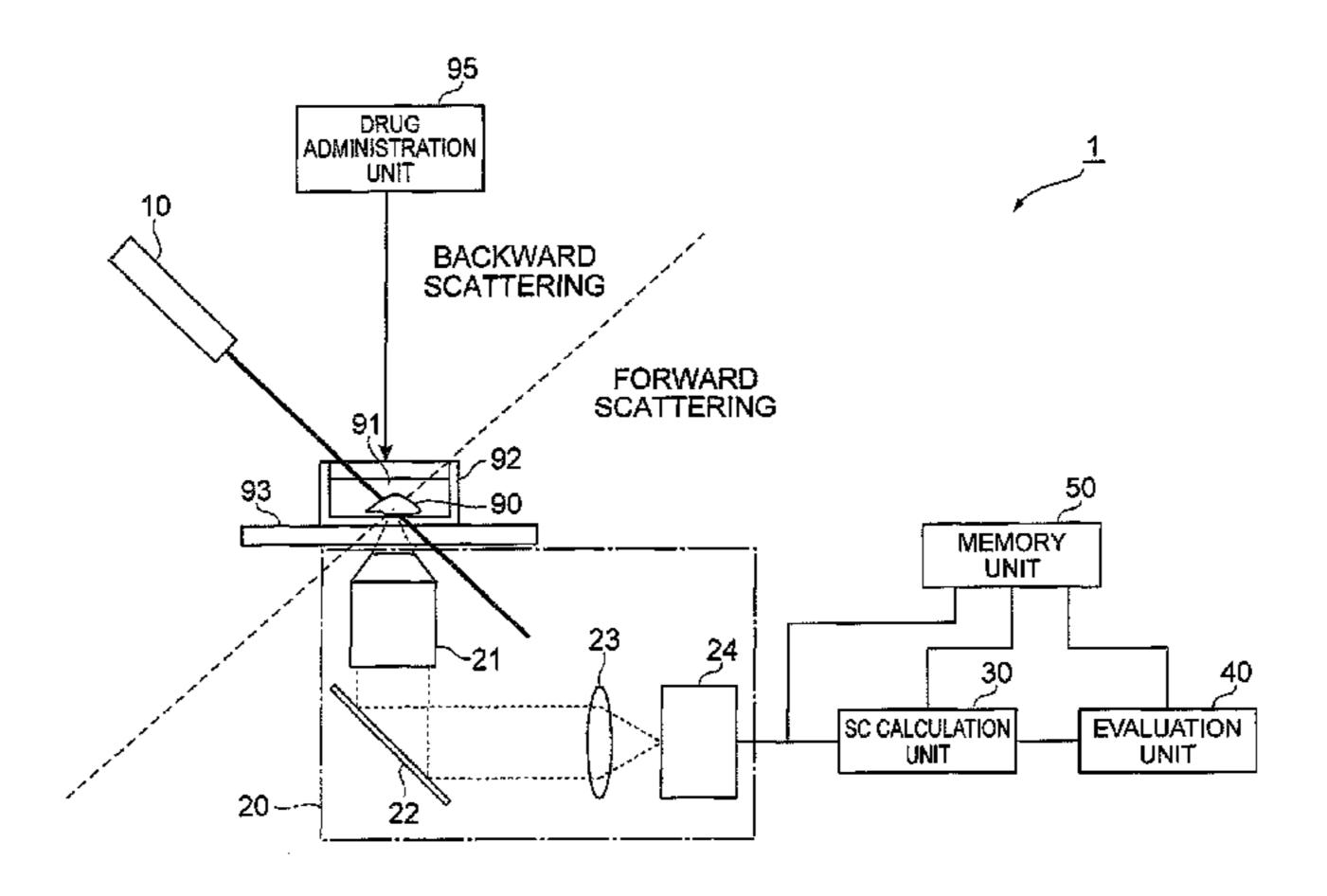
mum value  $K_{max}$  to obtain a normalized speckle contrast value  $K_n$ . The evaluation unit evaluates motion of the aggregated cells, based on the normalized speckle contrast value  $K_n$  at each time  $t_n$ .
