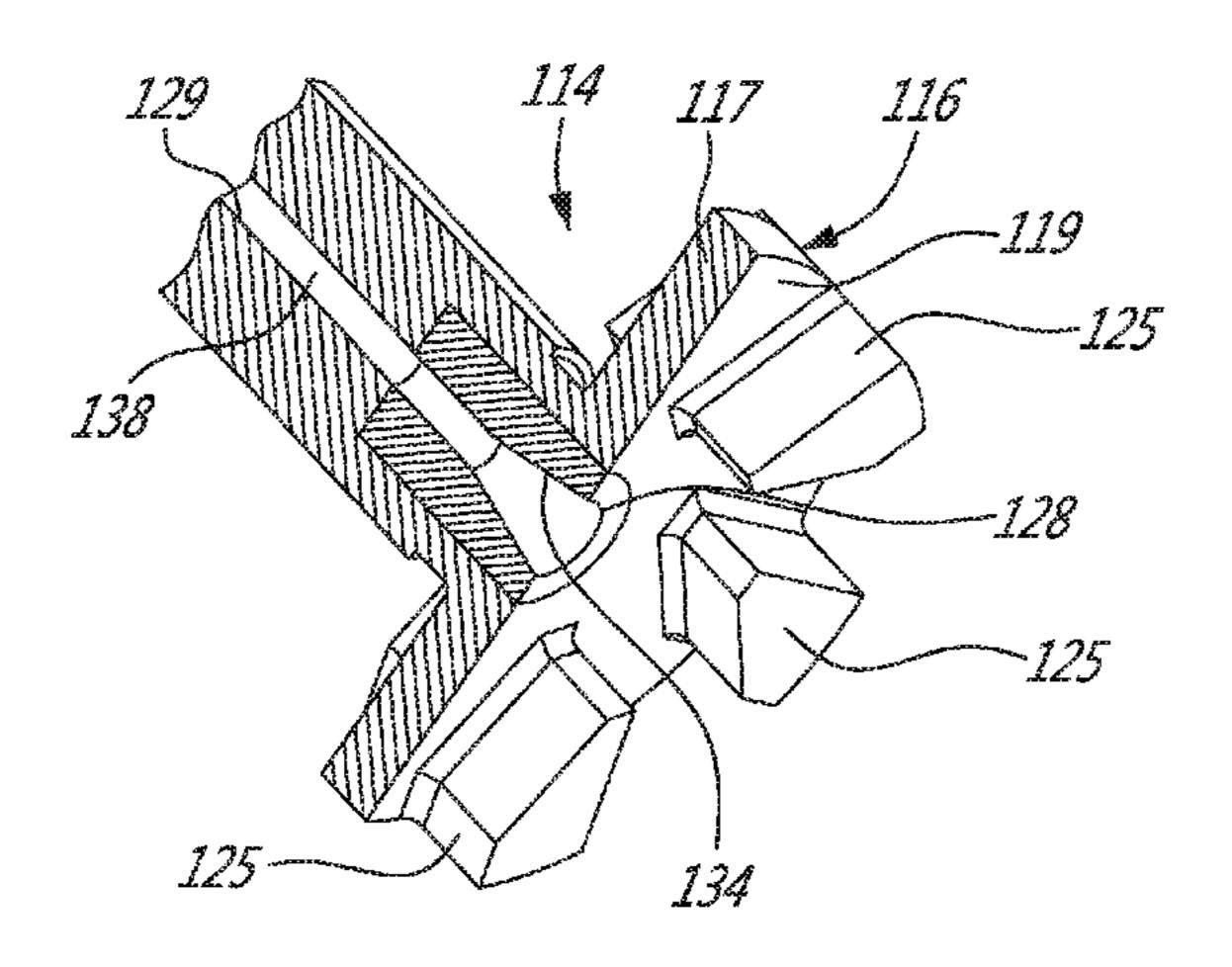
portion extending to an axial outlet, the discharge portion having a narrow end connecting the main portion of the supply conduit and a broader end at the axial outlet.
