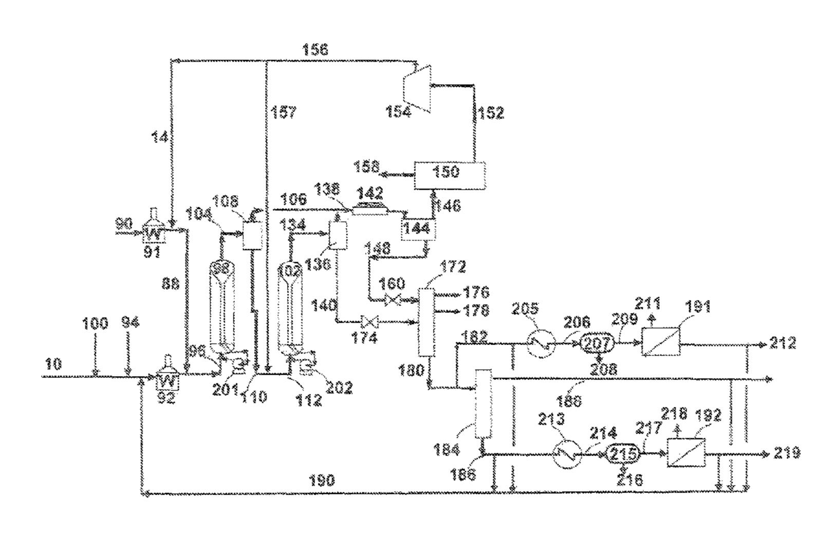
of separating the sediments from the heavy fraction originating from the maturation stage c) to obtain said heavy fraction.
