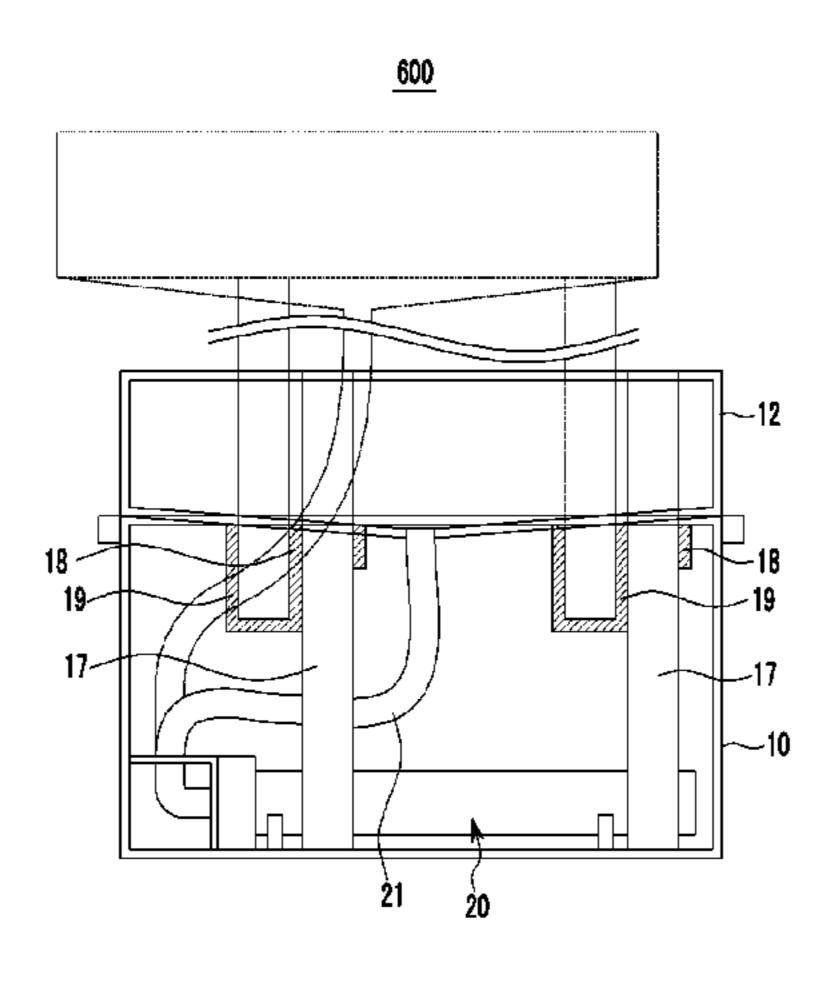
the water container through the hollow fiber membrane module, in which the hollow fiber membrane module causes the raw water supplied from the raw water supplying part collide with the hollow fiber membrane to move the hollow fiber membrane, so that it is possible to minimize contamination of the hollow fiber membrane, minimize use of energy using electricity, and wash the hollow fiber membrane by a physical method.
