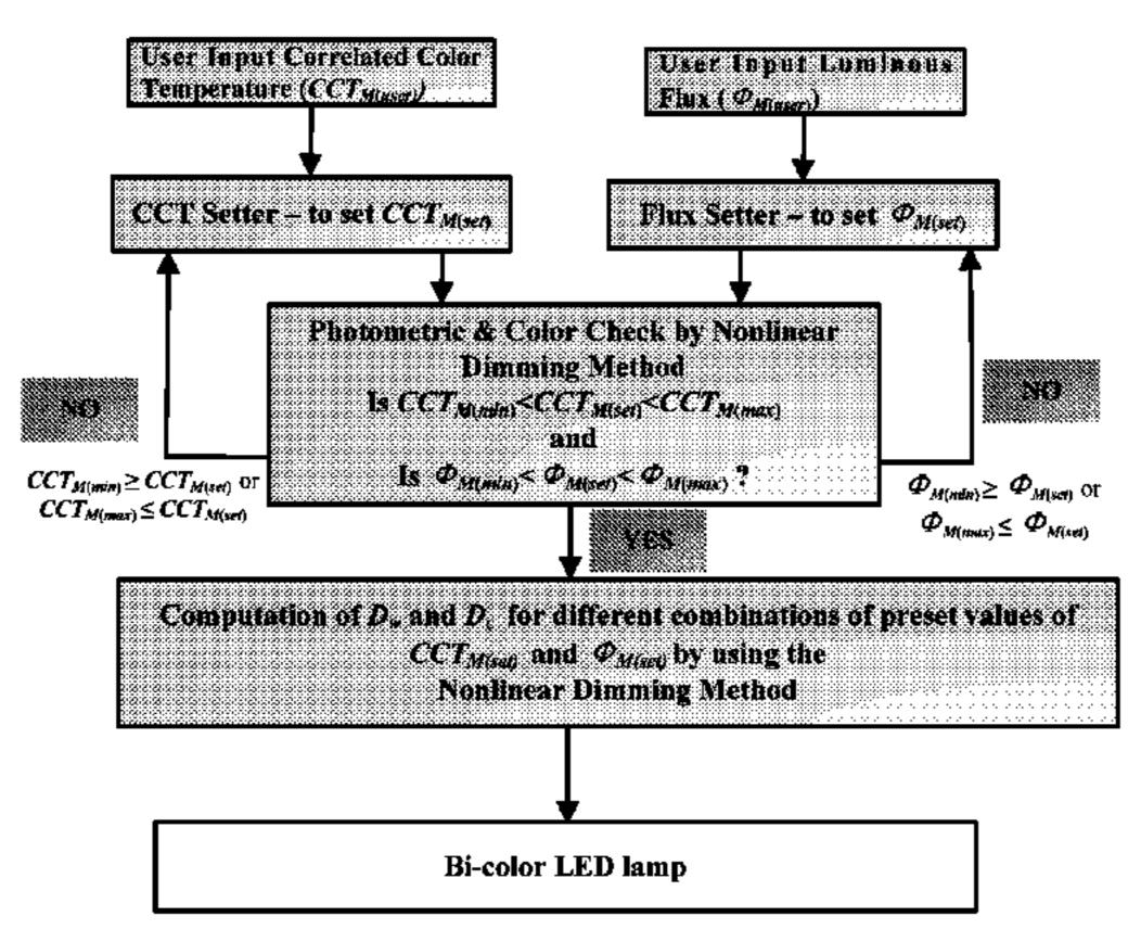
combined luminous flux for the LED lighting system (3, 4). An associated method is also provided.
