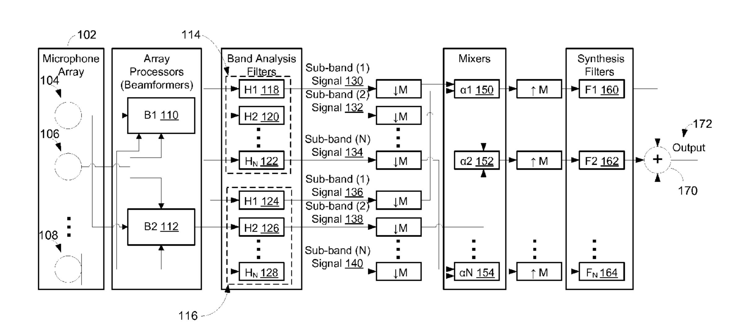
signal and generating a fourth output corresponding to the second sub-band based on the second microphone array processing signal. The method includes performing a first set of microphone mixing operations to generate an adaptive mixer output for the first sub-band and performing a different set of microphone mixing operations to generate another adaptive mixer output for the second sub-band.
