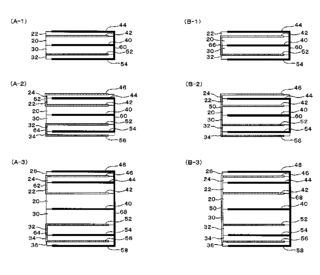
electric layers decrease gradually in an outward direction. A piezoelectric sound-generating body is constructed by affixing the piezoelectric driving element to a support plate and supporting the piezoelectric driving element with a frame.
