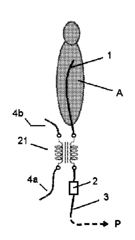
oscillator which is represented by the conductor (1, 3) by a damping element (4; 6) in order to prevent or limit RF heating of the examination object (A) at or surrounding the conductor (1, 3).
