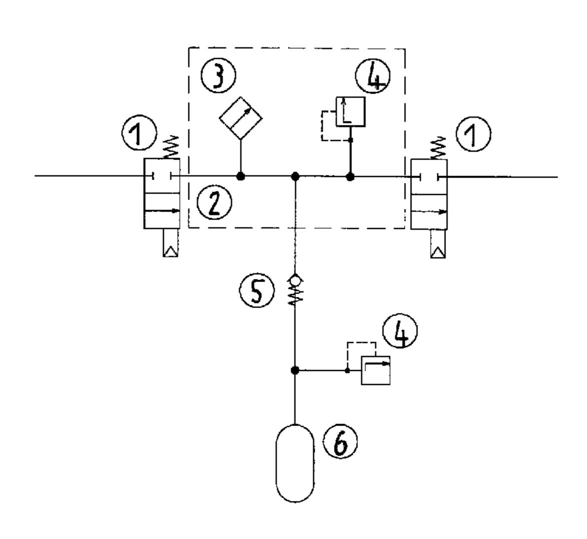
valve, wherein a leak detection diagnosis can be carried out by means of a pressure sensor that can be integrated.
