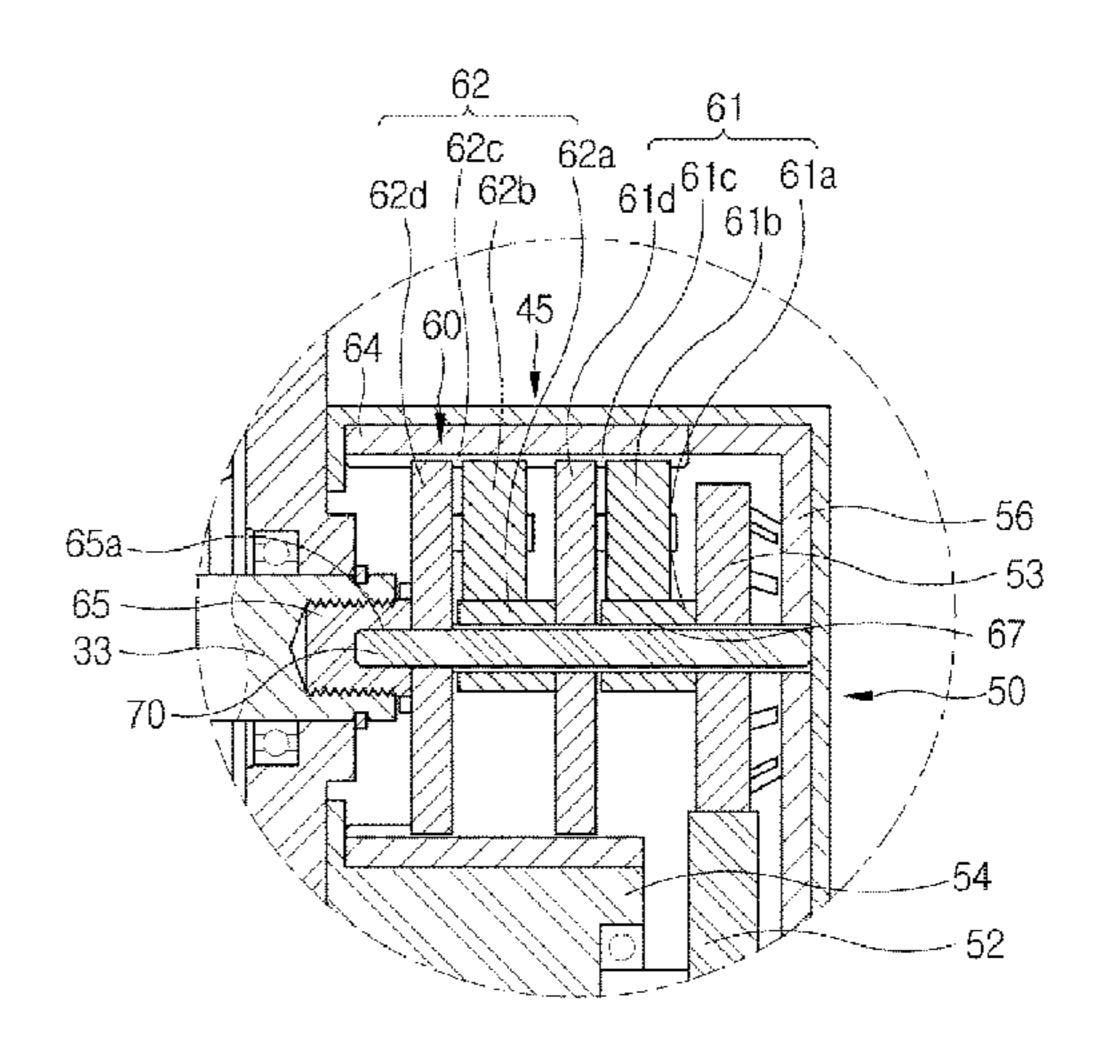
a rotational power, and an output shaft provided on the carrier and coupled to the spindle. The center pin has one end press-fitted and fixed to the output shaft.
