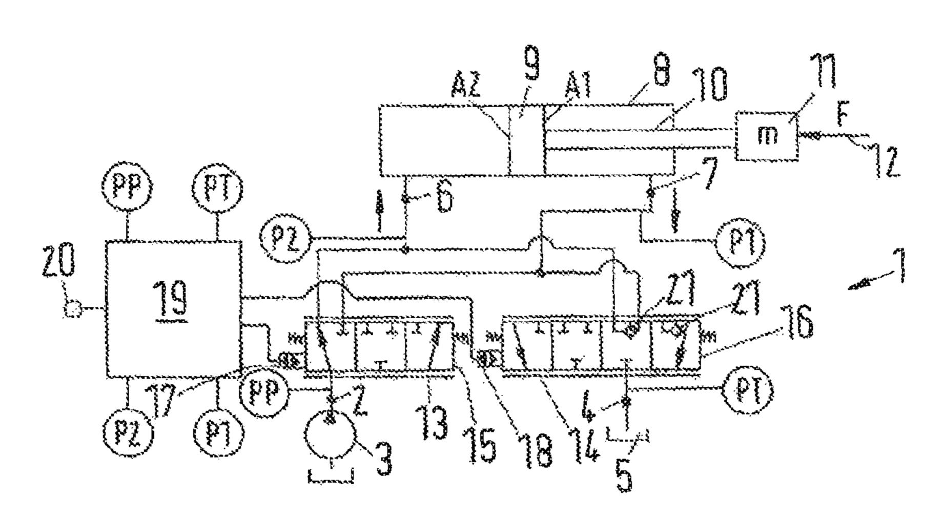
regenerative flow path when a feed pressure at said working port arrangement (6, 7) exceeds a predetermined pressure level.
