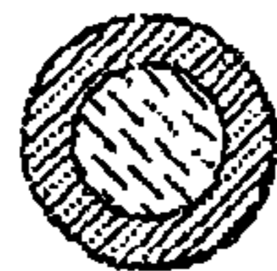
SPHERICAL METAL NANOSHELL COVERING DIELECTRIC SPHEROID CORE
