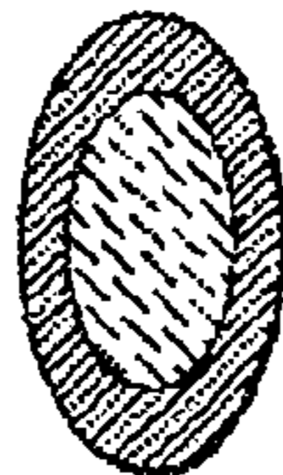
OBULATE METAL NANO- SHELL COVERING DIELEC- TRIC SPHEROID CORE
