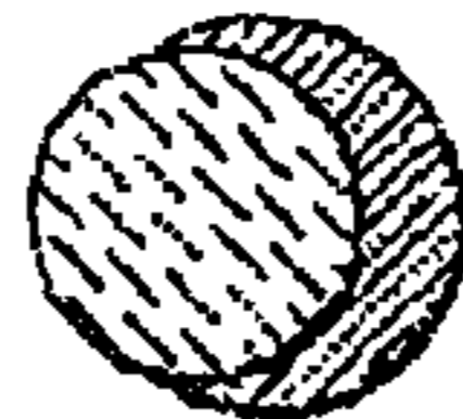
DIELECTRIC NANOPARTICLE CORE COVERED WITH METAL NANOCAP
