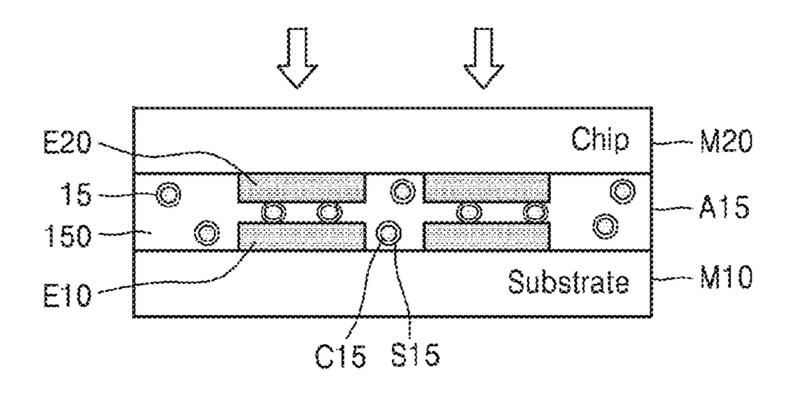
may include the core portion outflowed from the particle and may further include an intermetallic compound.
