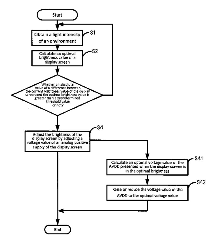
adjusted by adjusting a voltage value of an analog positive power supply of the display screen.
