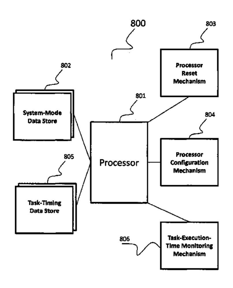
Limit for one or more tasks that are executed by the Processor, and [vi] a Task-Execution-Time Monitoring Mechanism (806) that is designed to monitor the execution time of tasks that are executed by the Processor and take corrective action, by means of the Processor Reset Mechanism (803) and the Processor Configuration Mechanism 804, if the task breaches its pre-determined Task WCET Limit or Task BCET Limit.
