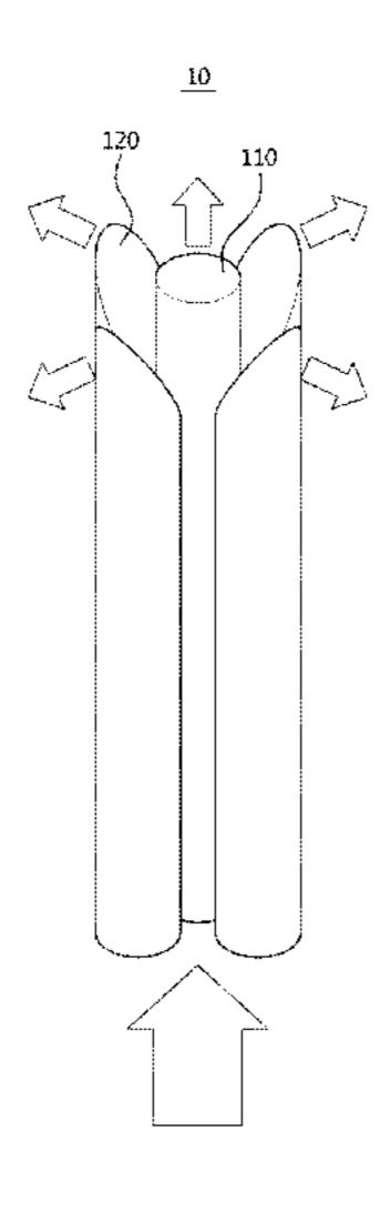
center thereof, the forward irradiation optical fiber having a flat end surface; and a side irradiation unit including a side irradiation optical fiber disposed at the periphery of the forward irradiation unit, the side irradiation optical fiber having an inclined end surface to laterally reflect a laser beam, wherein the forward irradiation unit and the side irradiation unit can be formed as a single bundle.
