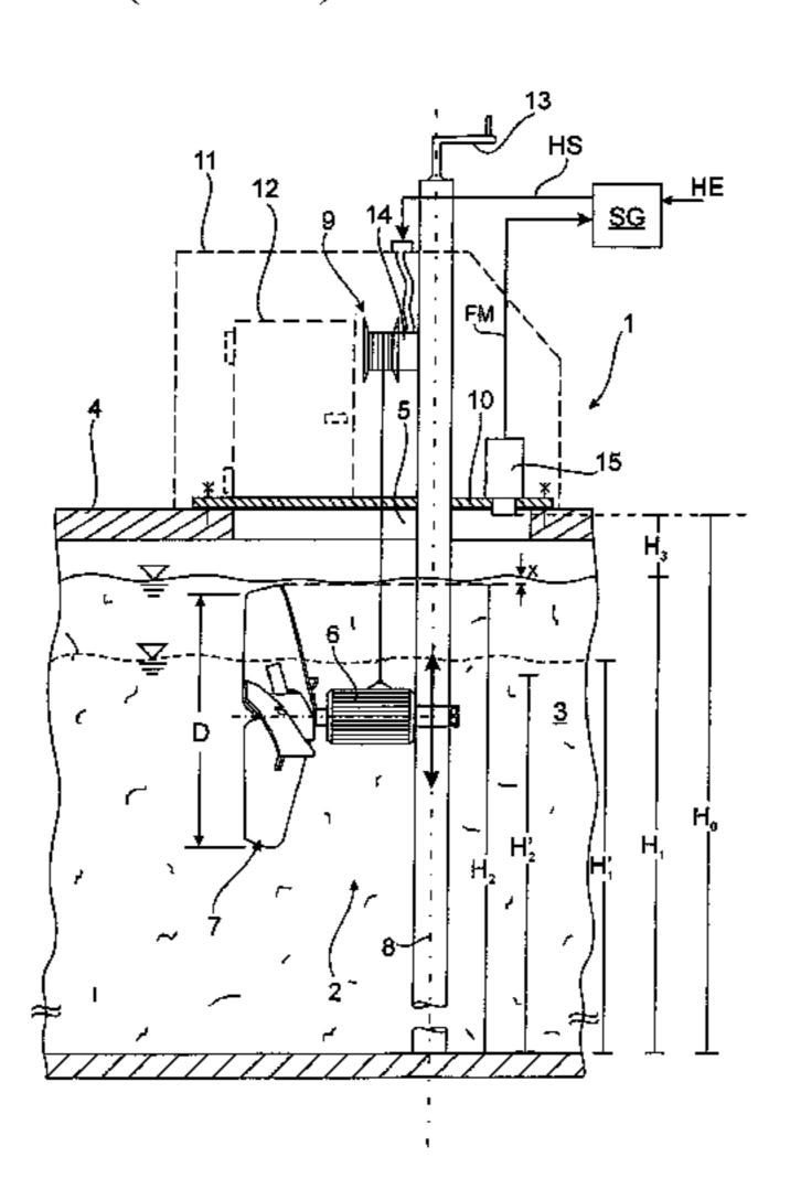
that the stirrer is lowered and the agitator blades continue to be fully immersed in the substrate.
