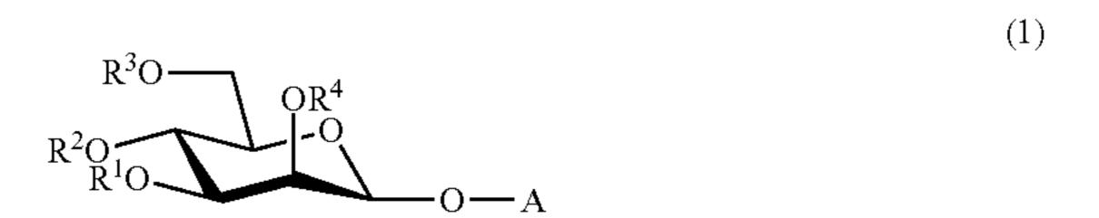
in the formula, R<sup>1</sup> to R<sup>4</sup> are the same as or different from each other and represent an alkanoyl group or a hydrogen atom, and A represents a sugar alcohol residue or a polyol residue.
