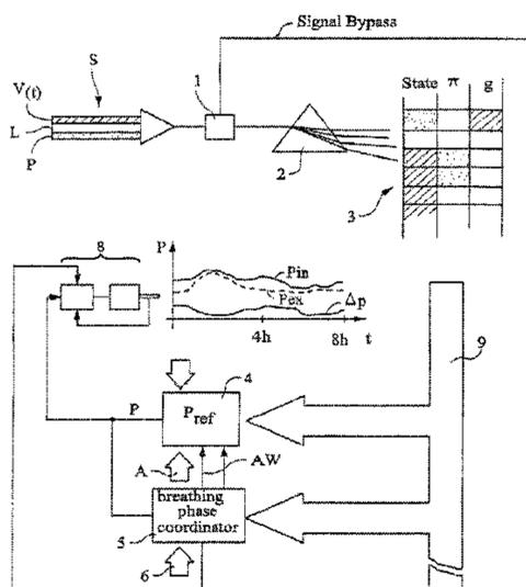
pressure signal generator is provided for generating the pressure control signal, taking into account determined data field entries which are at least selected by the extraction device.
