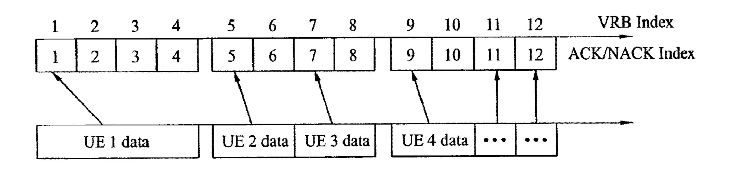
ACK/NACK signal for transmission data mapped to information of at least one of a virtual unit resource allocated to the transmission data and a virtual unit resource allocated to control information of the transmission data, and receives the ACK/NACK signal for the transmission data through the information of resources for receiving the ACK/NACK signal.
