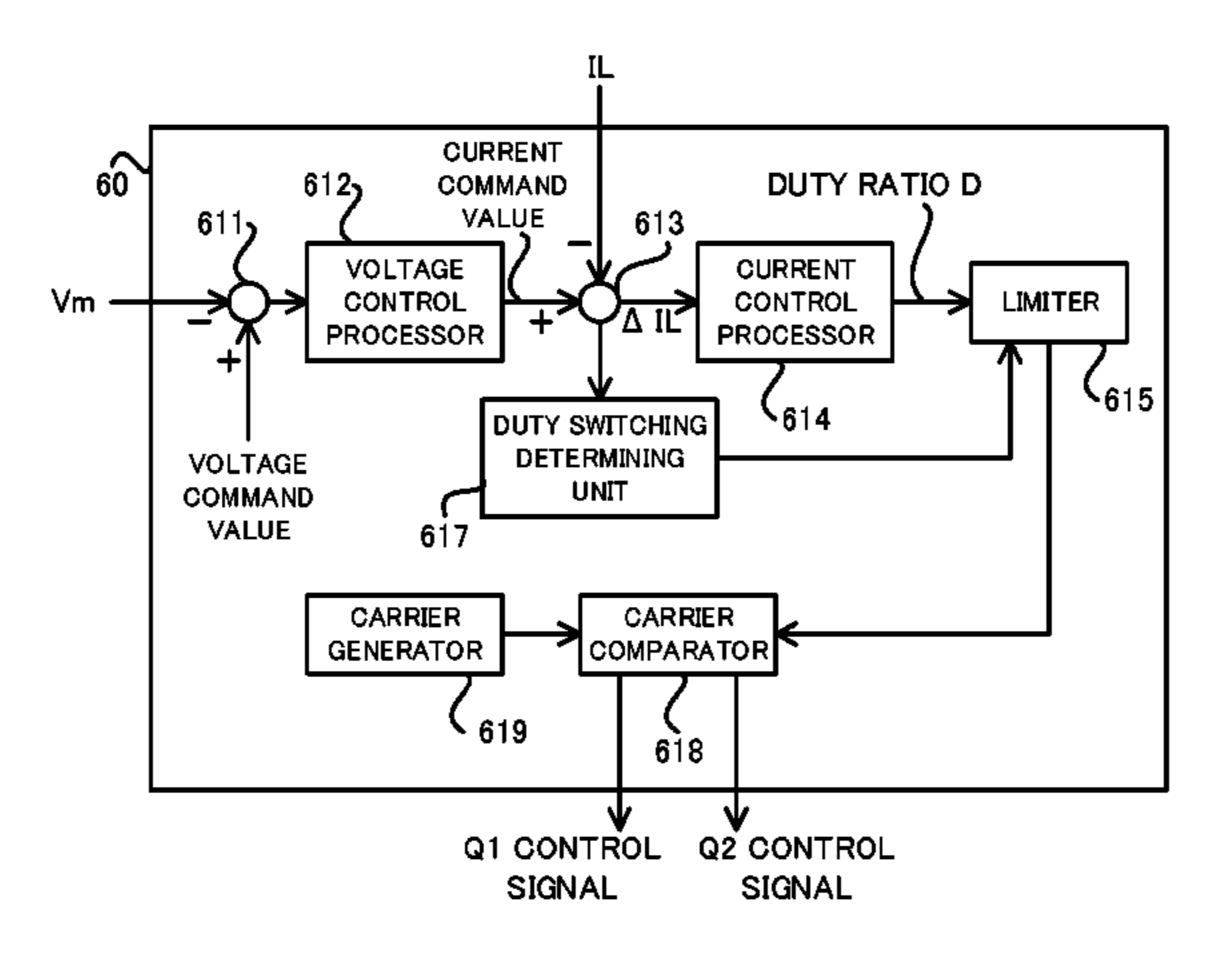
ing element to perform a switching control on the basis of the duty ratio which is calculated by the calculating device.
