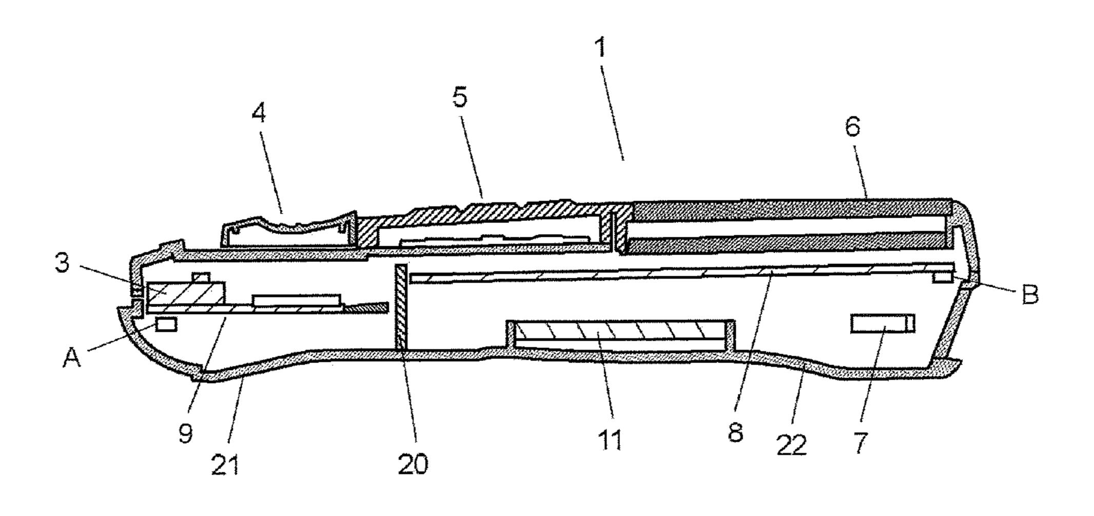
sors (A) and (B). Furthermore, a measurement value obtained by the measurement portion is corrected using temperature information from either one of the temperature sensors (A) or (B) that is provided in the end portion on the side where the temperature change is smaller.
