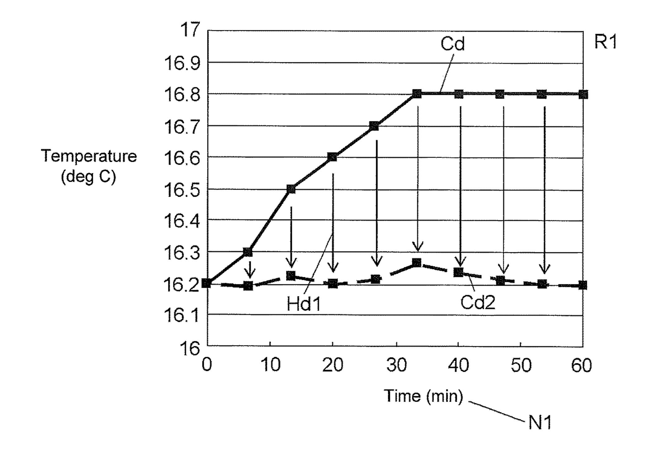
—■— Temperature sensor D ambient temperature 16 °C hand temperature 34 °C —■— Temperature sensor D after correction
