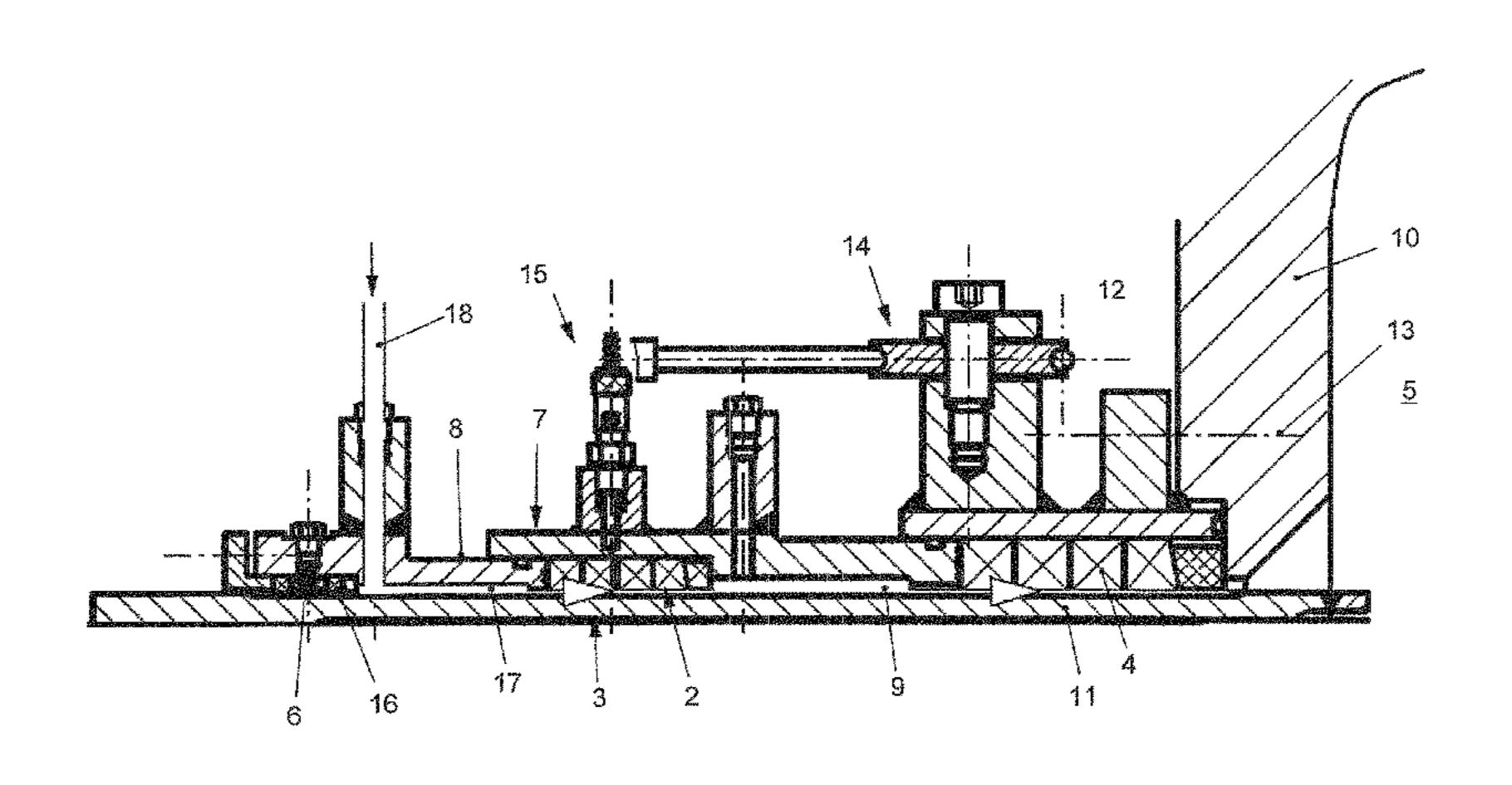
(7), is metered in here, the liquid, apart from a residual excess, being drawn into the dynamic seal (2) by a pressure difference therewithin and thereby forming an effective block and seal.
