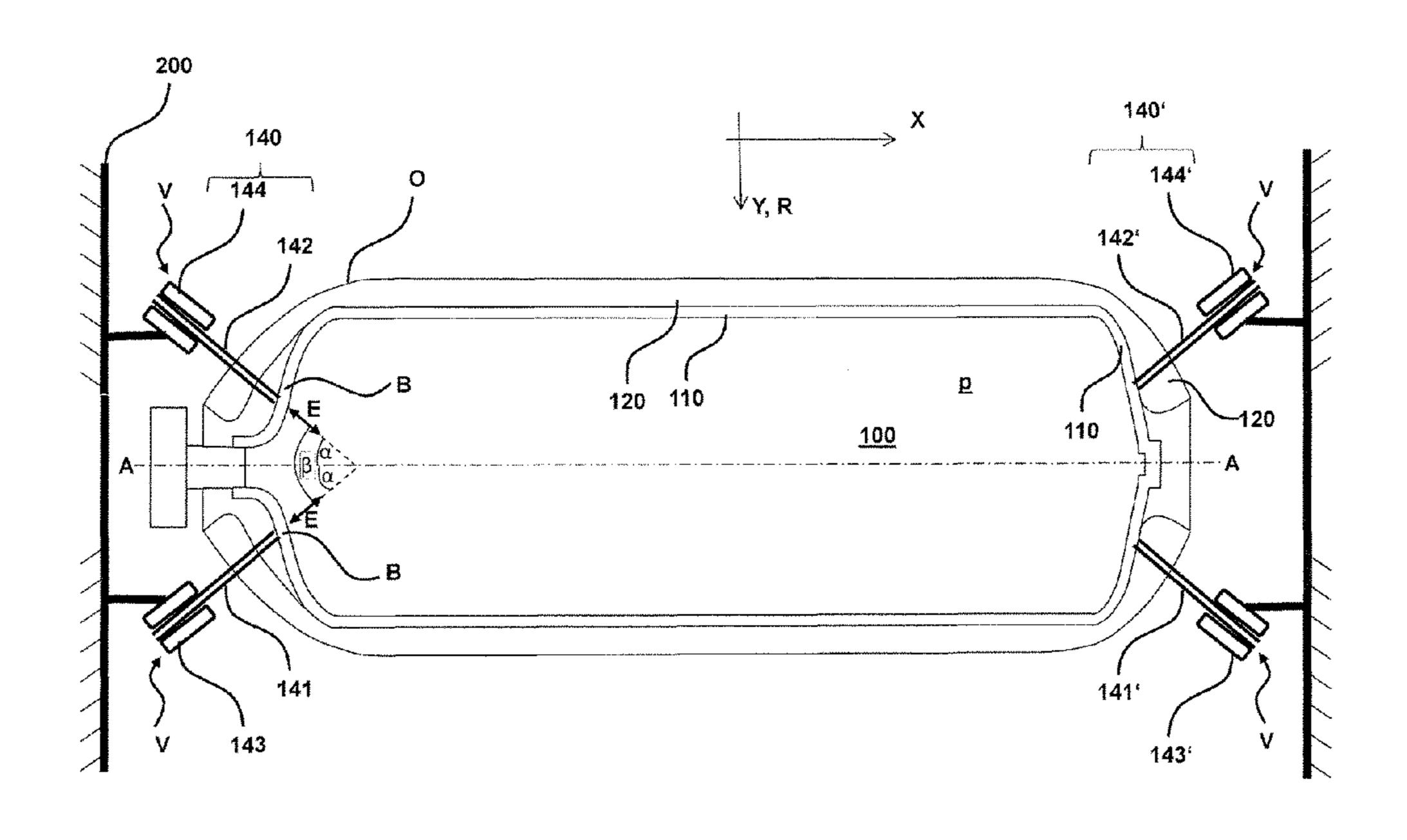
expansion. The connecting pin and the bearing are, in the connecting point, at least regionally shaped and arranged such that the expansion is kinetically guided with only one translational degree of freedom by way of a movement of the bearing and/or of the connecting pin.
