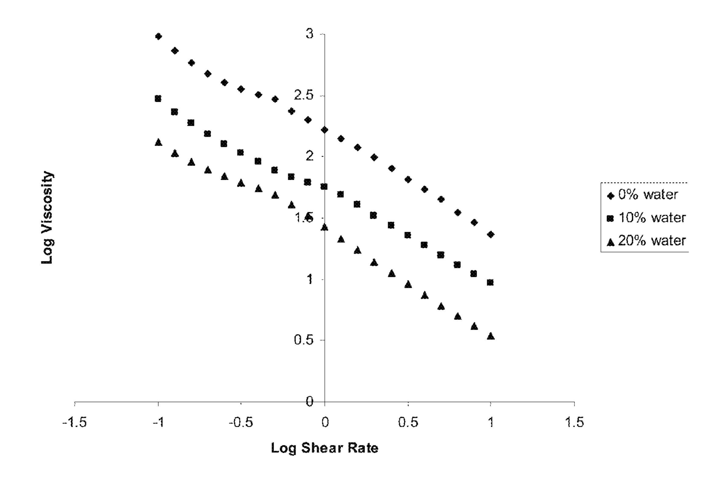
Fig. 2: Rheological profile of a regular guar gum formulation with the addition of 10% and 20% water. Each value is the average of at least 5 replicates ( $n \ge 5$ ).
