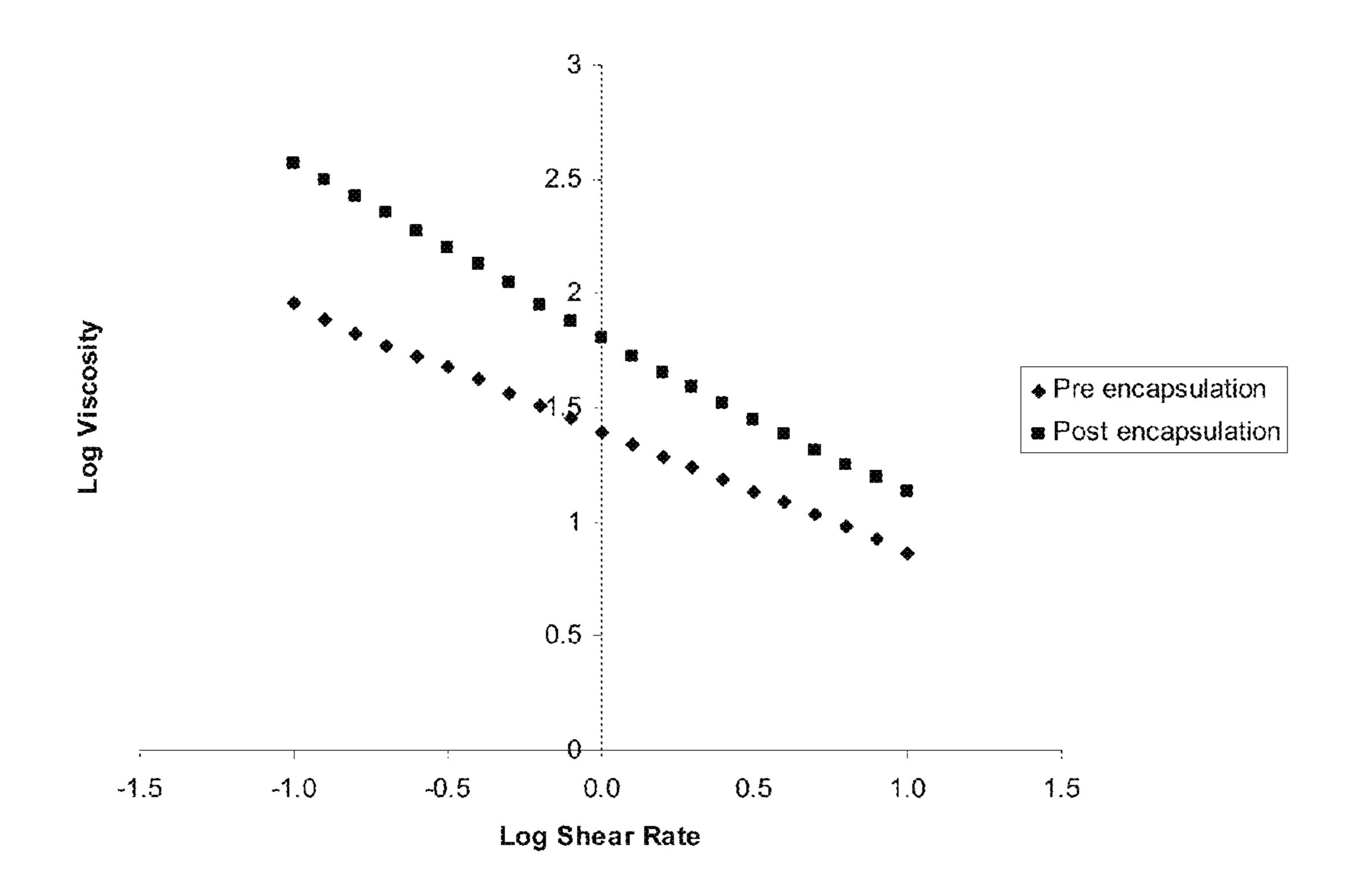
Fig. 6: Rheological profile of a modified guar gum/ PEG 400 fill formulation of an embodiment of the present invention after storage.
