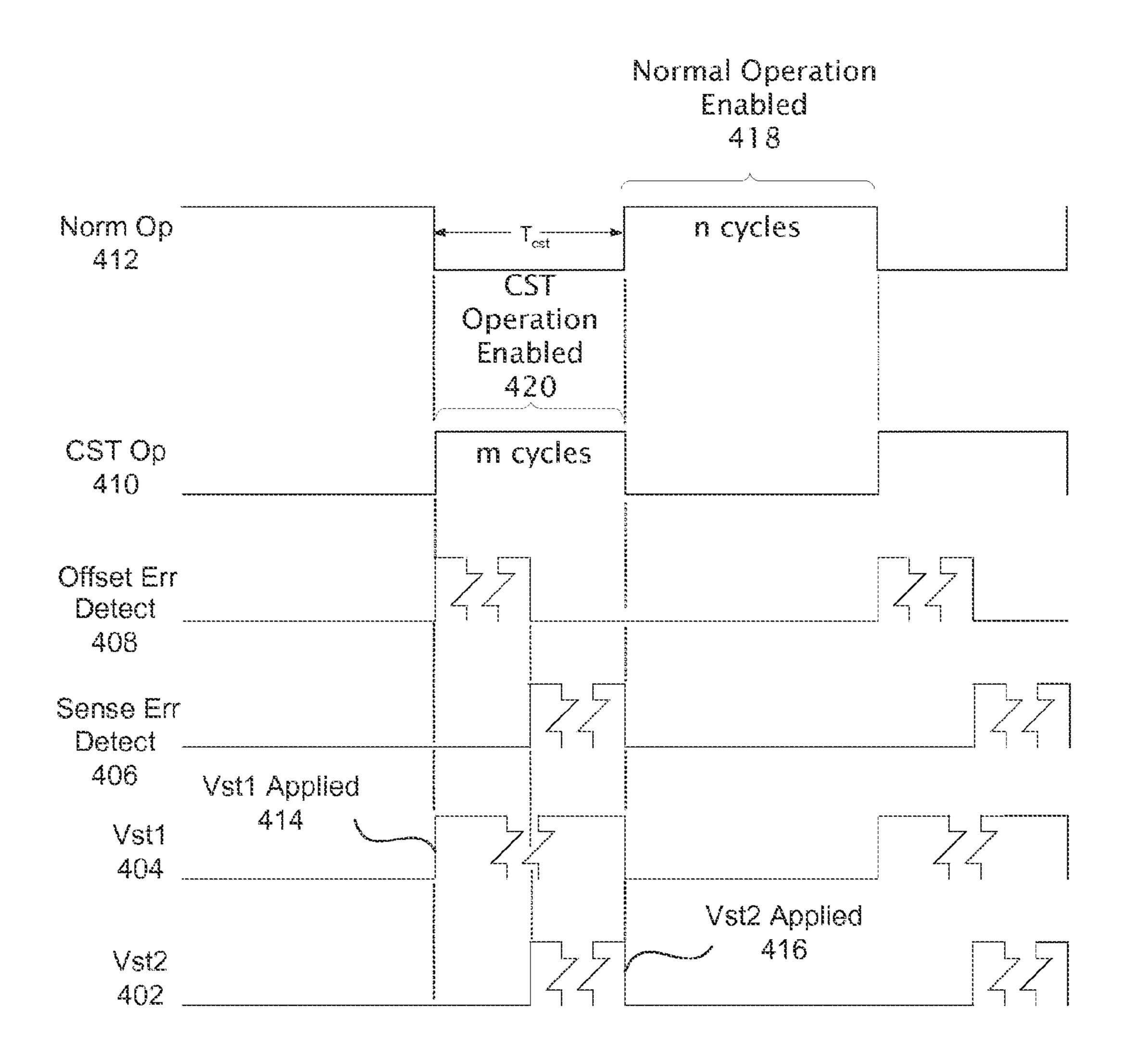
Timing Diagram for Method of implementing CST 400
