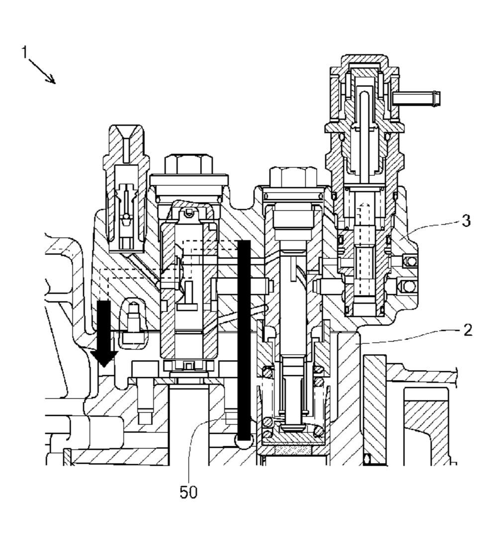
prevented from being unable to start in the state that dew condensation occurred in the fuel injection pump and froze.
