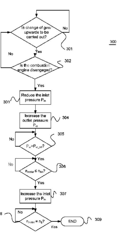
combustion gas is reduced, to increase the pressure at the outlet by constriction of the exhaust gas flow, and when the rate of revolution of the combustion engine (101) has at least partially fallen towards a second rate of revolution, to control the turbocharger unit such that the combustion gas pressure is increased. Also a system and a vehicle including the system.
