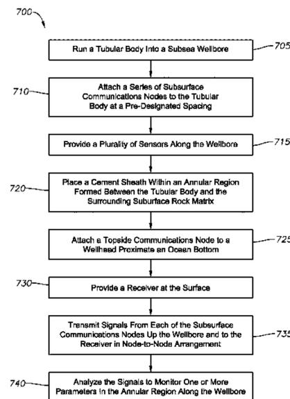
wellbore at high data transmission rates for data indicative of a parameter within an annular region behind the string of casing. A method of evaluating a parameter within an annular region along a cased-hole wellbore is also provided herein. The method uses a plurality of data transmission nodes situated along the casing string which send signals to a receiver at the surface. The signals are then analyzed.
