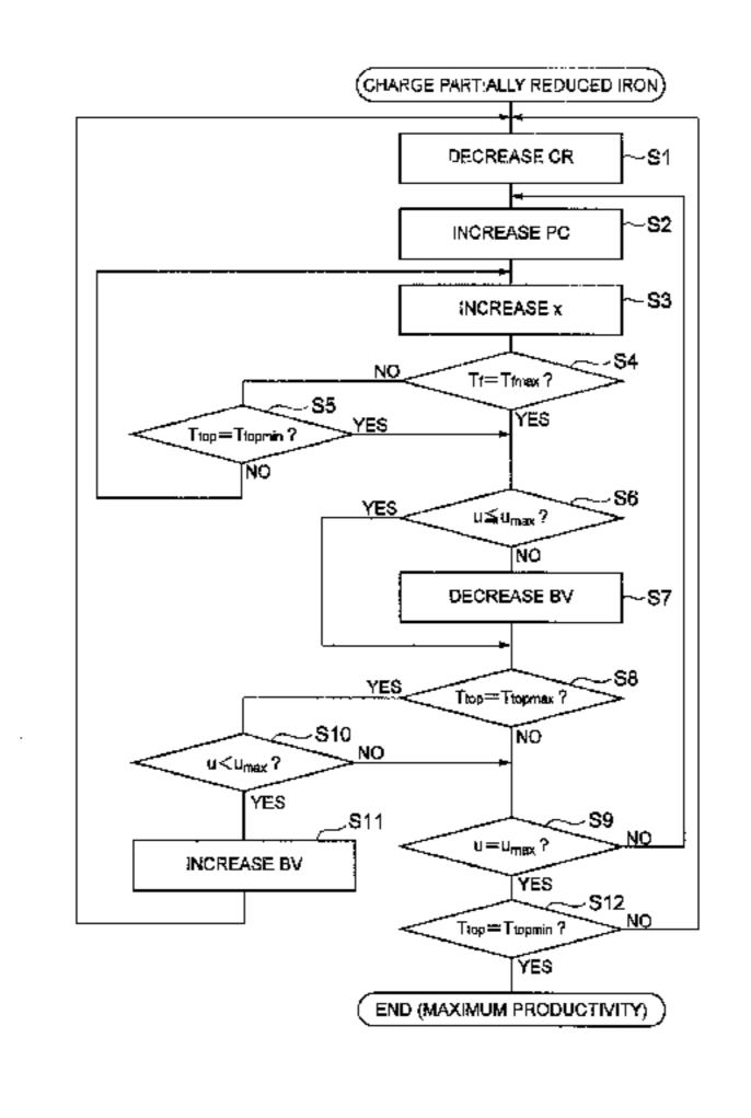
monitoring a tuyere combustion temperature  $T_f$  and the furnace-top temperature  $T_{top}$ ; and a fourth step of determining whether an injection rate of the oxygen-enriched air needs to be adjusted, based on a value of the in-furnace superficial gas velocity u.
